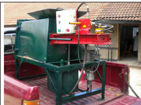
Fig. 4: A manufactured Compactor Prototype
