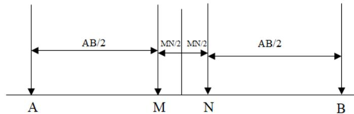
Figure 3: Schlumberger VES configuration (Kearey et al. 2002).
