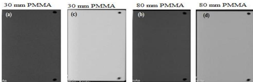
Figure 3: Mammograms obtained by irradiating PMMA phantoms of different thicknesses.
