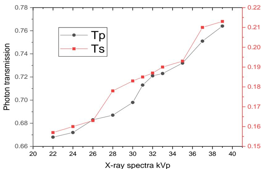
**Figure 5:** The relationship between the transmission of photons (primary and scatter) versus the X-ray spectra (kVp) through a 20 mm PMMA phantom thickness.
