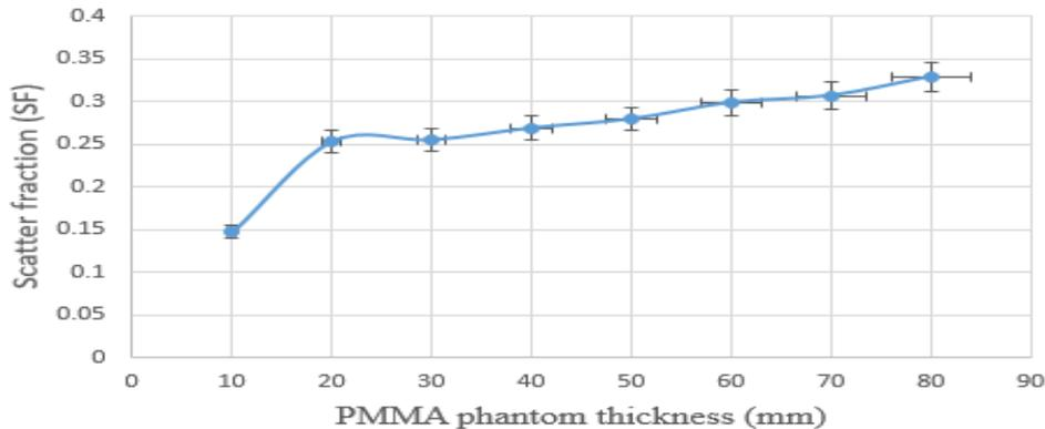
**Figure 4** The scatter fraction (SF) against PMMA phantom thickness at a fixed spectral kVp.
