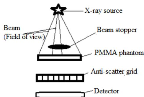
**Figure 1:** Experimental set-up of the imaging geometry.
