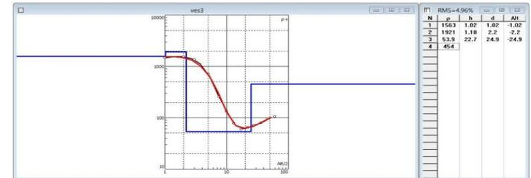
Figure 6: Resistivity curve for VES 3(004°38'27.3"N, 008°28'43.7"E).
