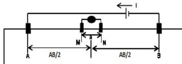
**Figure 3:** A Schematic representation of the Schlumberger Array.
