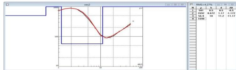
Figure 5: Resistivity curve for VES 2(004°38'28.9"N, 008°29'11.2"E).
