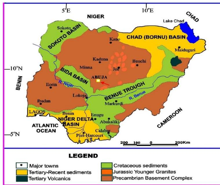
**Figure 2:** Generalized geological map of Nigeria showing the three lithological units (After: Obaje 2009a, b).
