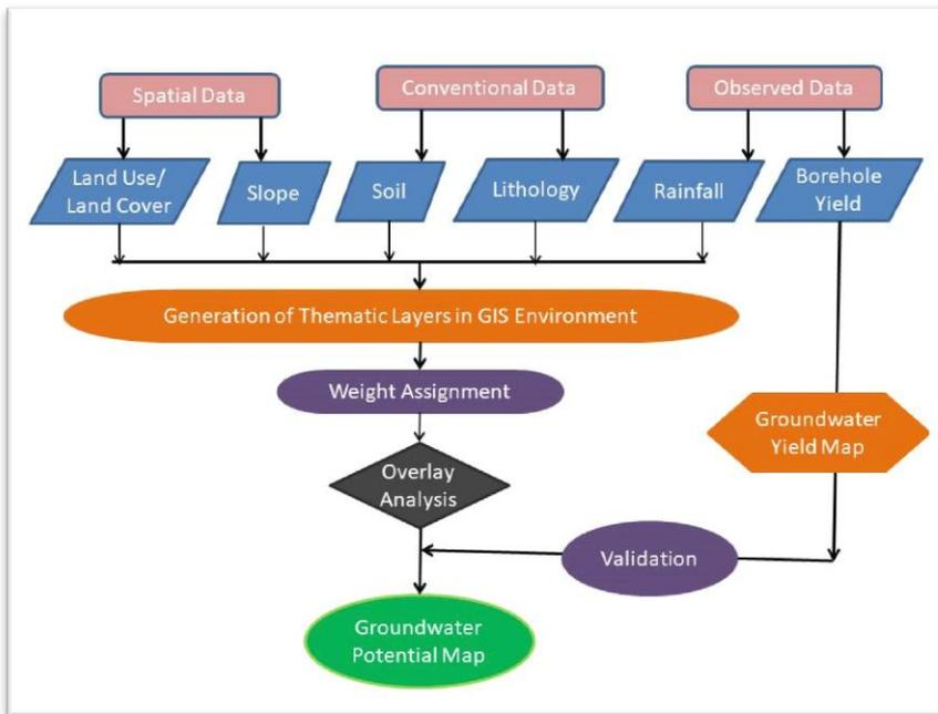
**Figure 2:** Flow chart for generating groundwater potential map.
