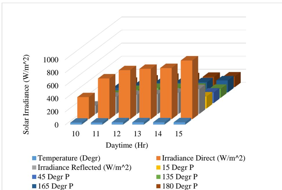
**Figure 7:** Solar irradiance and PV power output dataset for 15°, 45°, 135°, 165° and 180°.
