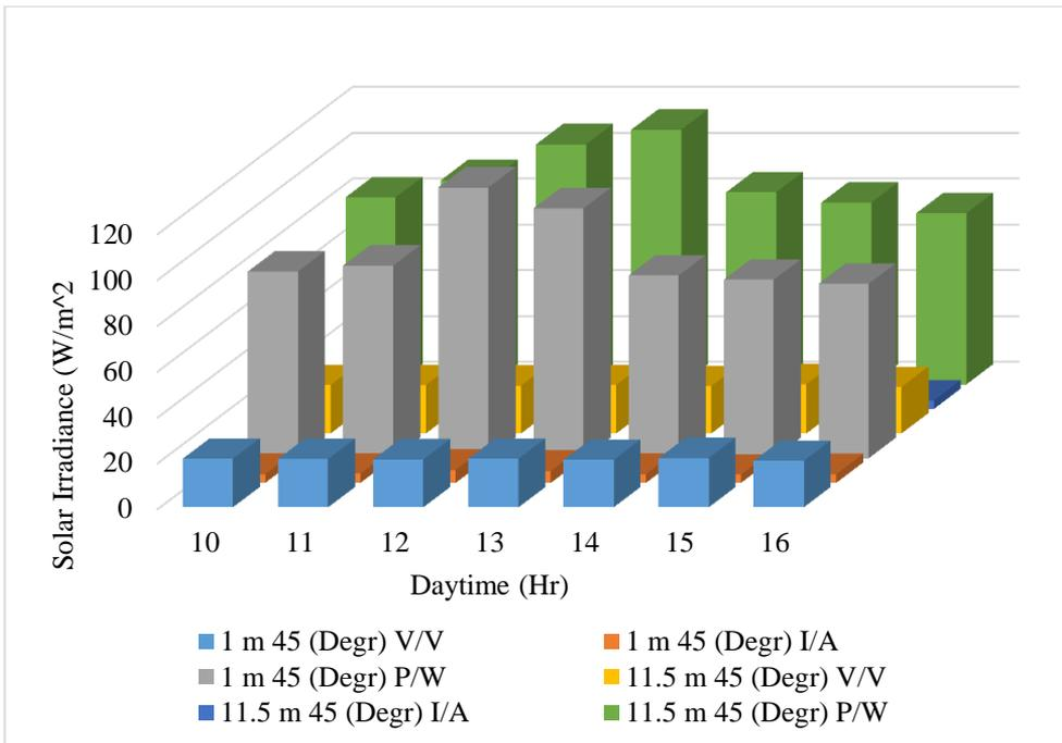
**Figure 6b:** Comparison of voltage, current, and power datasheet for 45° tilt angle at 1 m and 11.5 m.
