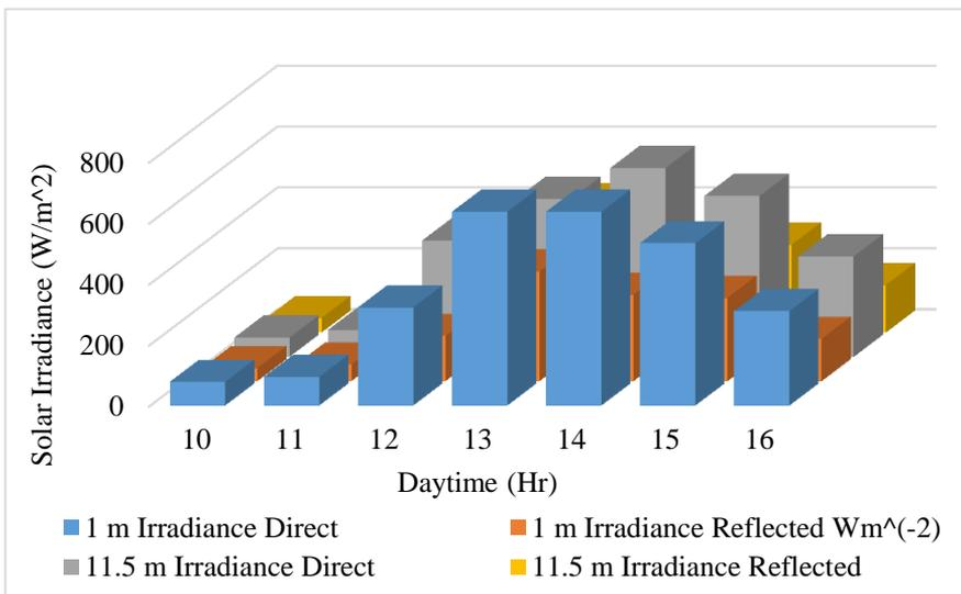
**Figure 4:** Comparison of direct and reflected irradiance on a clear sky day at 1 m and 11.5 m.
