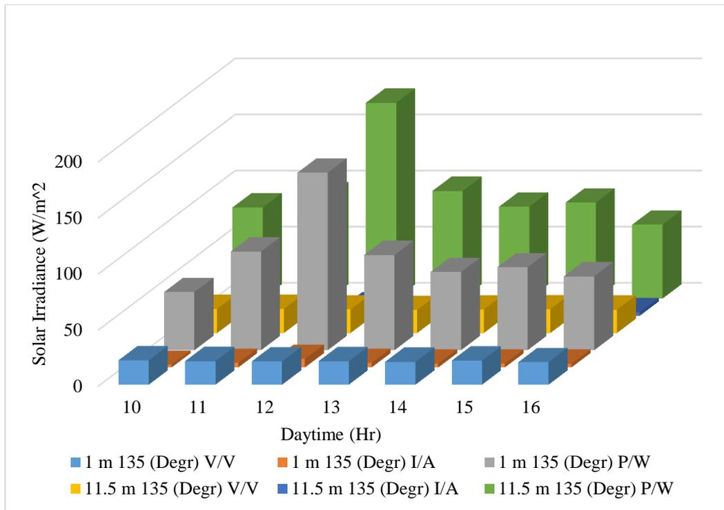
**Figure 6c:** Comparison of voltage, current, and power datasheet for 135° tilt angle at 1 m and 11.5 m (V = Voltage in Volts; I = Current in Ampere, A; P = Power in Watts, W).
