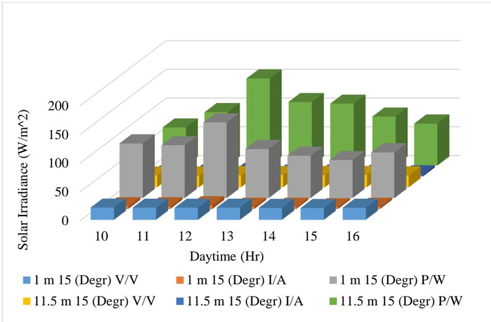
**Figure 6a:** Comparison of voltage, current, and power datasheet for 15° tilt angle at 1 m and 11.5 m.
