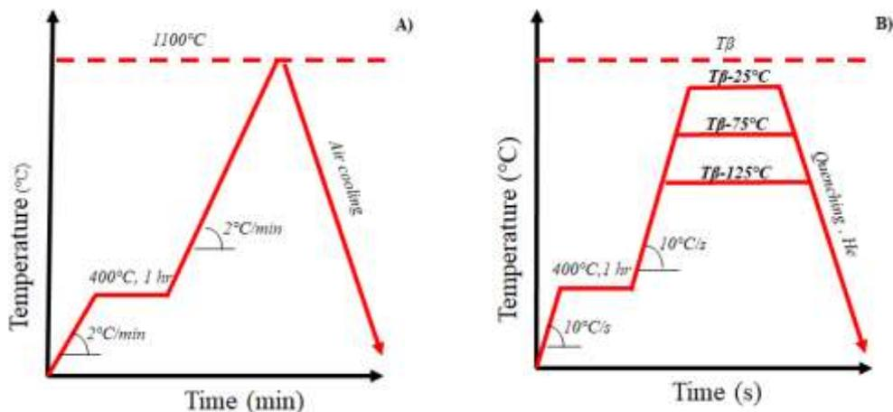
**Figure 3:** Sketch of heat treatment cycles: a) determination of transus temperature and b) isothermal holding at different temperatures
