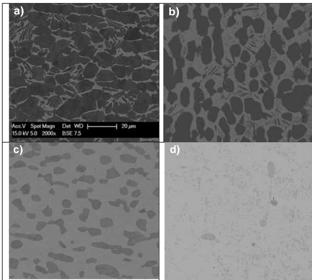
**Figure 8:** Typical microstructures of Ti54M alloy for as-received and after isothermal holding for 1 hour and subsequent quenching: a) as-received, b) 840°C, c) 890°C, d) 940°C
