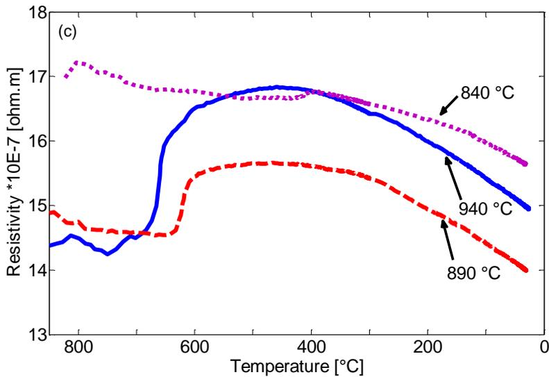
**Figure 6:** Evolution of electrical resistivity during heat treatment cycle: a) heating, b) isothermal holding, c) quenching.
