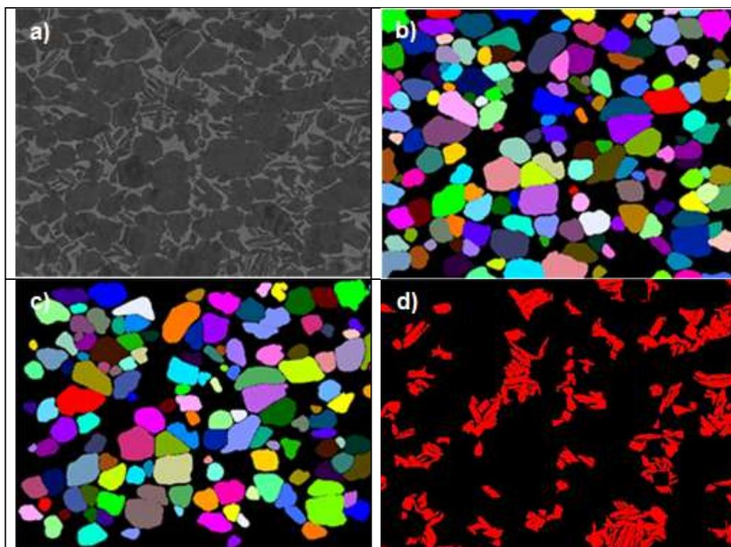
**Figure 4:** Image analysis after isothermal holding: (a) initial SEM image, (b) determining of  $\alpha$ -nodules phase fraction, (c) determination of density and size distribution of  $\alpha$ -nodules, and (d) determination of  $\alpha$ -lamellae phase fraction
