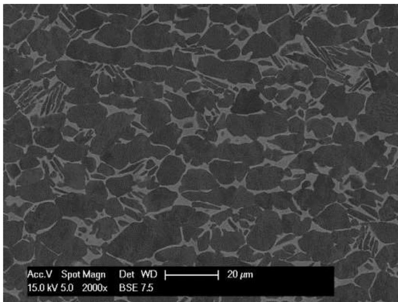
**Figure 1:** Initial microstructure of the as-received sample (*white:  $\beta$ -phase and grey:  $\alpha$ -phase*)
