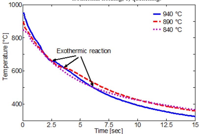
**Figure 7:** Variation of temperature with time during quenching.
