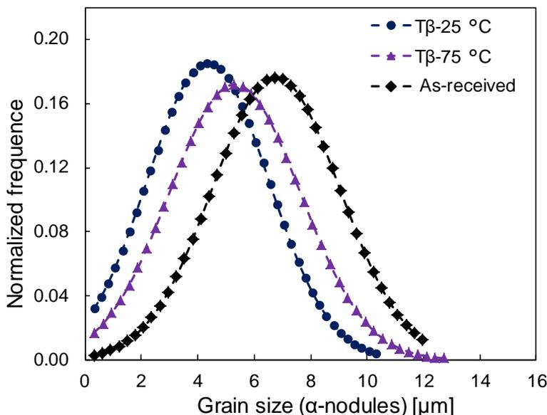
Figure 9: Distributions of  $\alpha$ -nodule grain size for different holding temperatures
