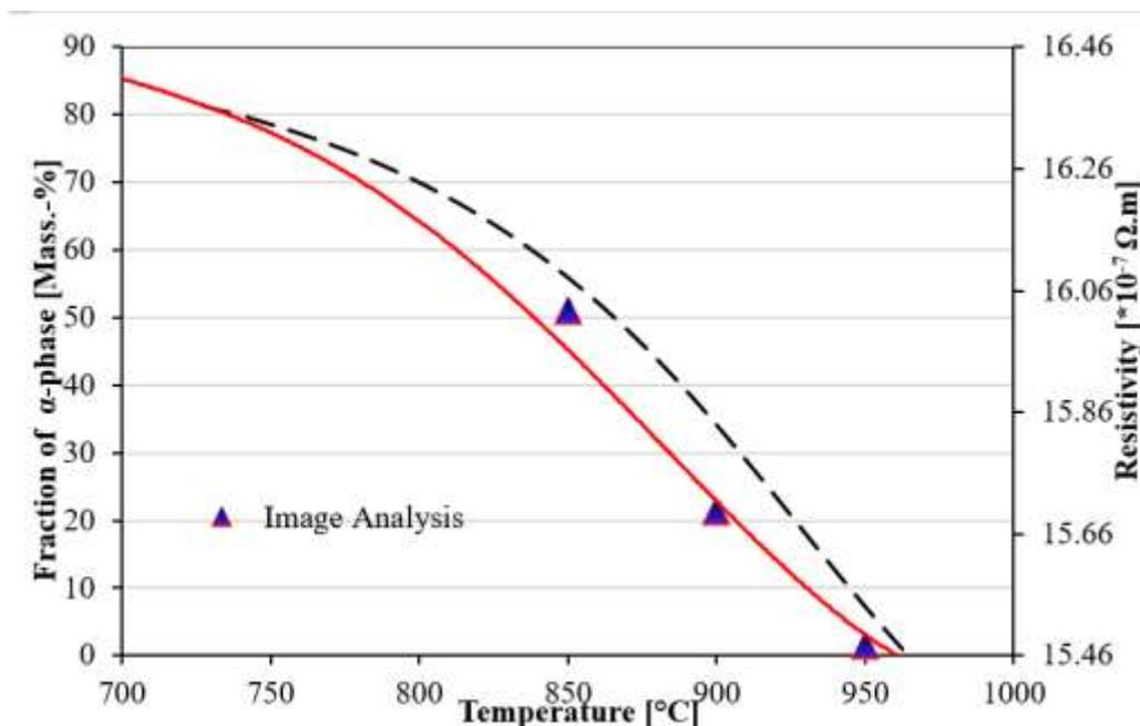
Figure 10: Variation of fraction of  $\alpha$ -phase and resistivity as a function of temperature.
