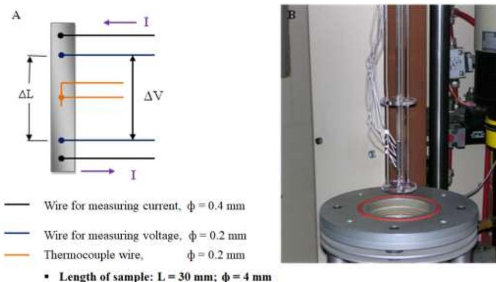
**Figure 2:** A) Sketch of the sample indicating principles of a “four-points” method and -B) experiment set-up for dilatometry experiment
