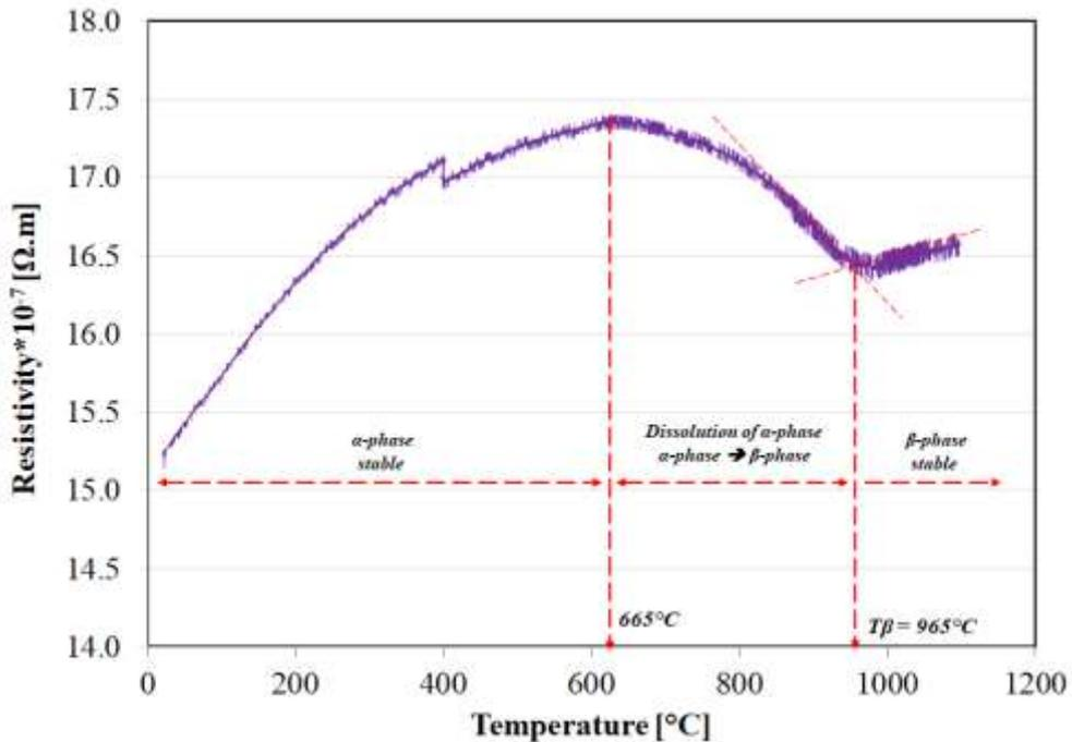
**Figure 5:** Determination of transus temperature ( $T_{\beta}$ ) for Ti54M
