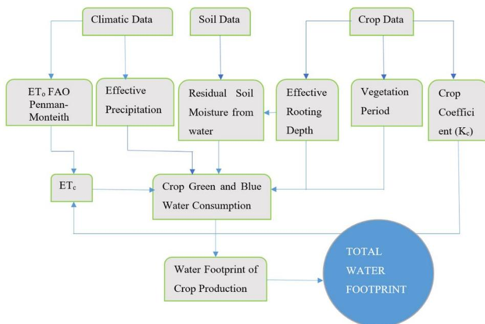
**Figure 3:** Flow diagram for calculation of water footprint of major crops in Wami/Ruvu basin (Adopted and modified from Yerli and Sahin 2022).
