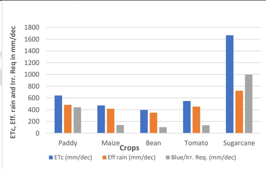
**Figure 5:** Crop evapotranspiration ( $ET_c$ ), effective rainfall (Eff rain) and blue/irrigation water requirements (Irr. Req) in mm/dec for Major crops grown in Wami/Ruvu Basin.
