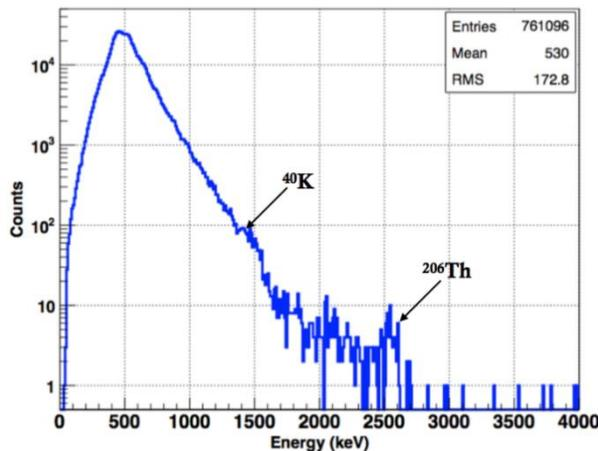
**Figure 6:** The background photon energy spectrum taken for ten hours.
