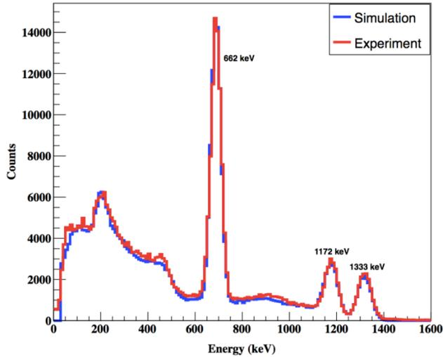
**Figure 8:** Comparison of experimental and simulated results using standard gamma-ray sources.
