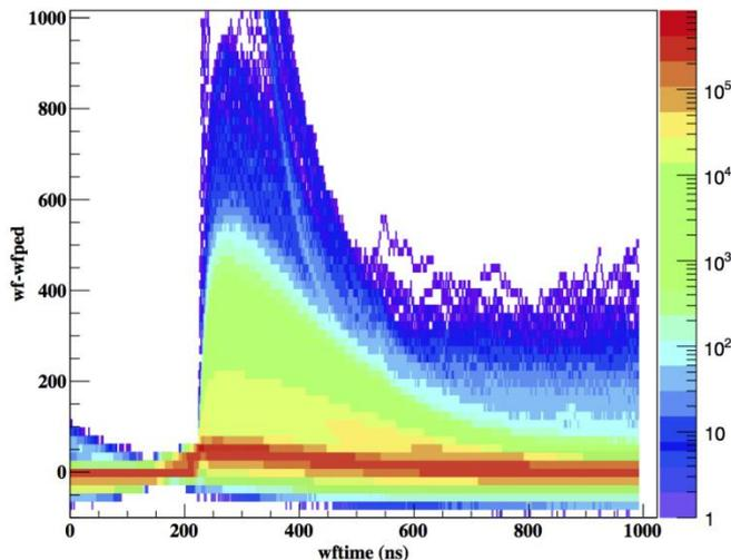
**Figure 4:** Superimposed NaI(Tl) detector signals digitized using a NKFADC500.
