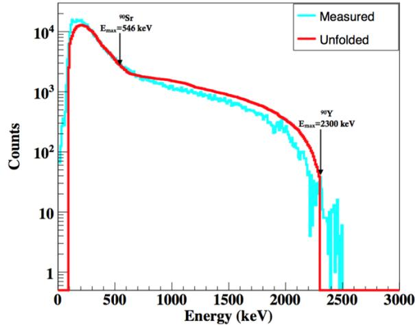
**Figure 10:** Measured spectrum of a  $^{90}\text{Sr}$  source (Cyan) and unfolded spectrum (Red) using the matrix inversion method.
