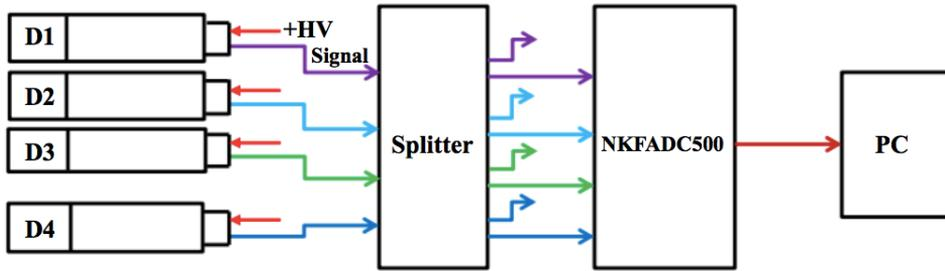
**Figure 3:** Schematic of an electronic data readout showing the signal from each detector.
