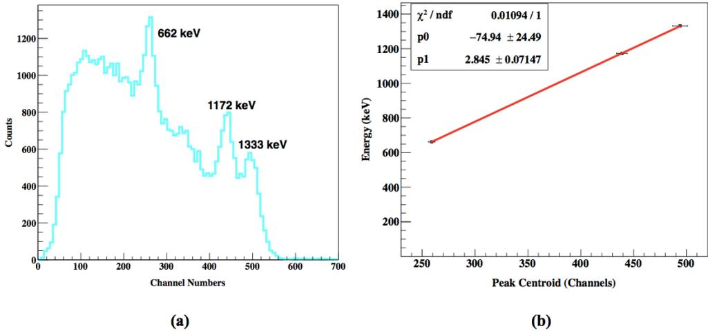
**Figure 5:** (a) The gamma-ray spectrum of  $^{137}\text{Cs}$  and  $^{60}\text{Co}$  used for energy calibrations. (b) The energy calibrations for the detectors D1 were used, and all fittings were done using the polynomial function of order one.
