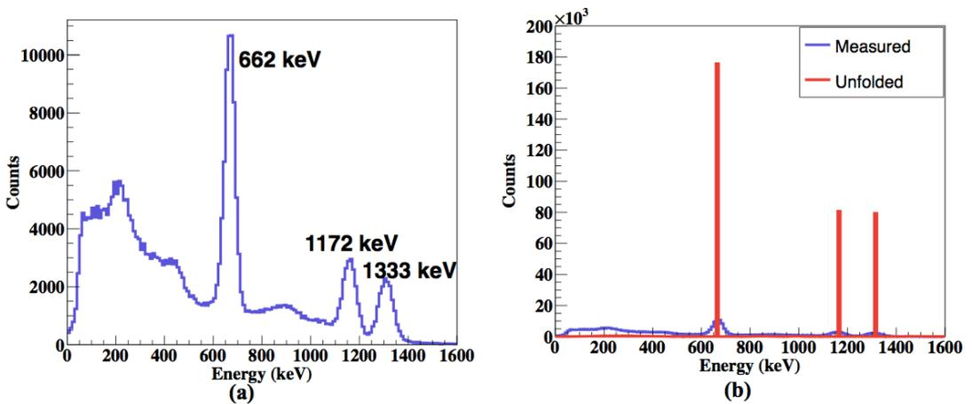
**Figure 9:** Measured energy spectrum of  $^{60}\text{Co}$  and  $^{137}\text{Cs}$  and deconvoluted spectrum (Red histogram) using the matrix inversion method.
