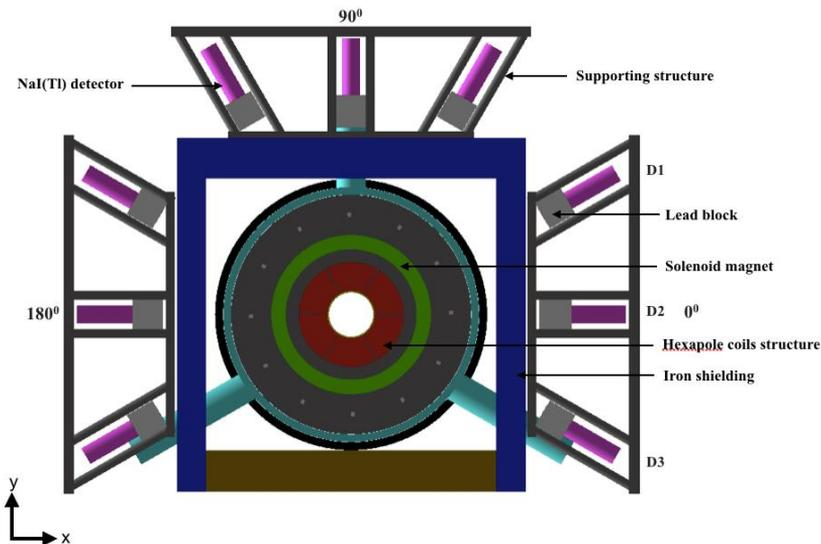
**Figure 2:** The schematic view of the nine NaI(Tl) detectors at the extraction side.
