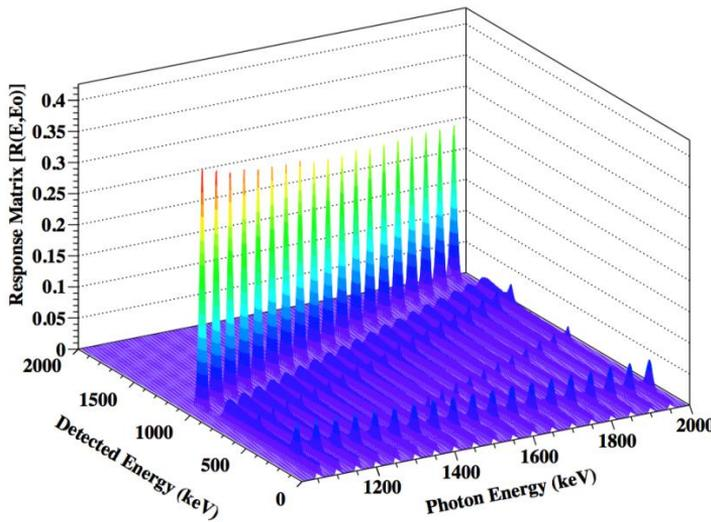
**Figure 7:** Simulated response function from various mono-energetic gamma rays using NaI(Tl) scintillation detector in 2D.
