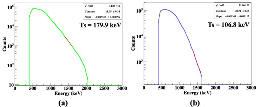
**Figure 12:** The spectral temperature calibrated from the detector D1 of the sample data measured at angle  $150^\circ$  (a) and  $330^\circ$  (b).
