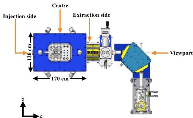
**Figure 1:** Schematic view of the low-energy accelerator facility at Busan Center of KBSI.
