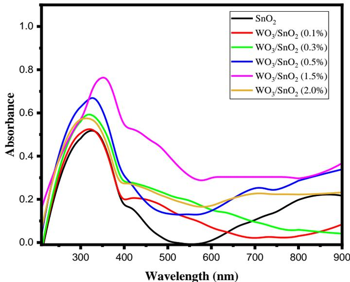
**Figure 3:** Absorbance as a function of wavelength for pure  $\text{SnO}_2$  and  $\text{WO}_3/\text{SnO}_2$  thin films with different proportions of  $\text{WO}_3$ .
