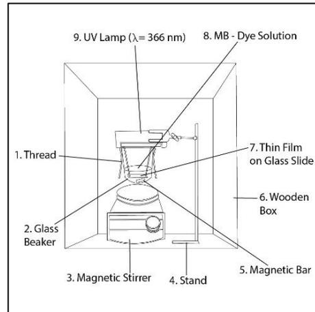
**Figure 1:** The experimental set-up that was used for the photocatalytic experiment.
