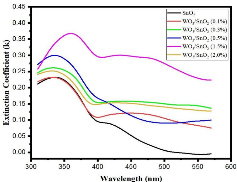
**Figure 6:** Extinction coefficient ( $k$ ) as a function of wavelength for pure  $SnO_2$  and  $WO_3/SnO_2$  thin films with different proportions of  $WO_3$ .
