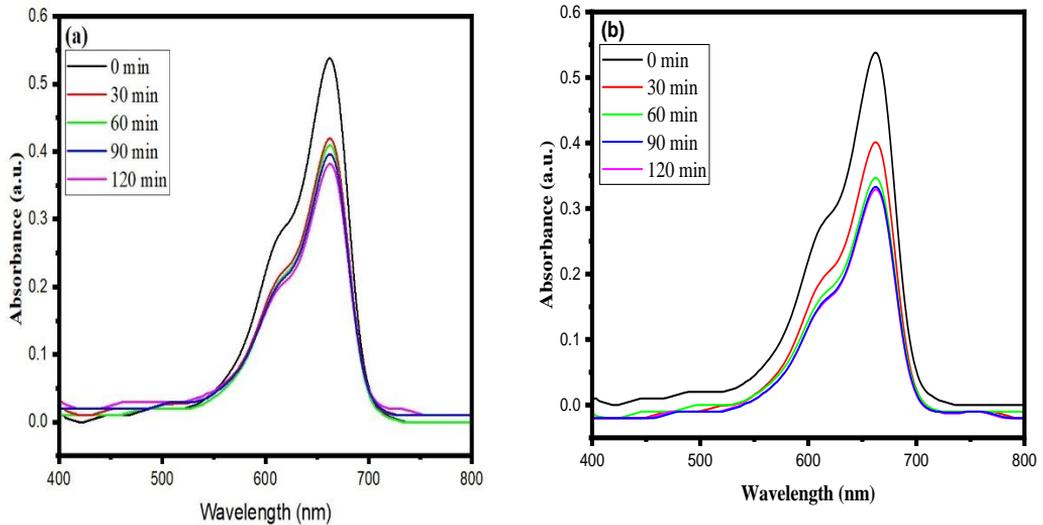
**Figure 8:** Absorption spectra of methylene blue for (a)  $\text{SnO}_2$  and (b)  $\text{WO}_3/\text{SnO}_2$  (1.5%) films.
