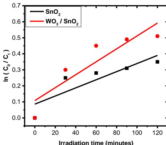
Figure 9: Plot of  $\ln(C_0/C_t)$  vs Irradiation time.
