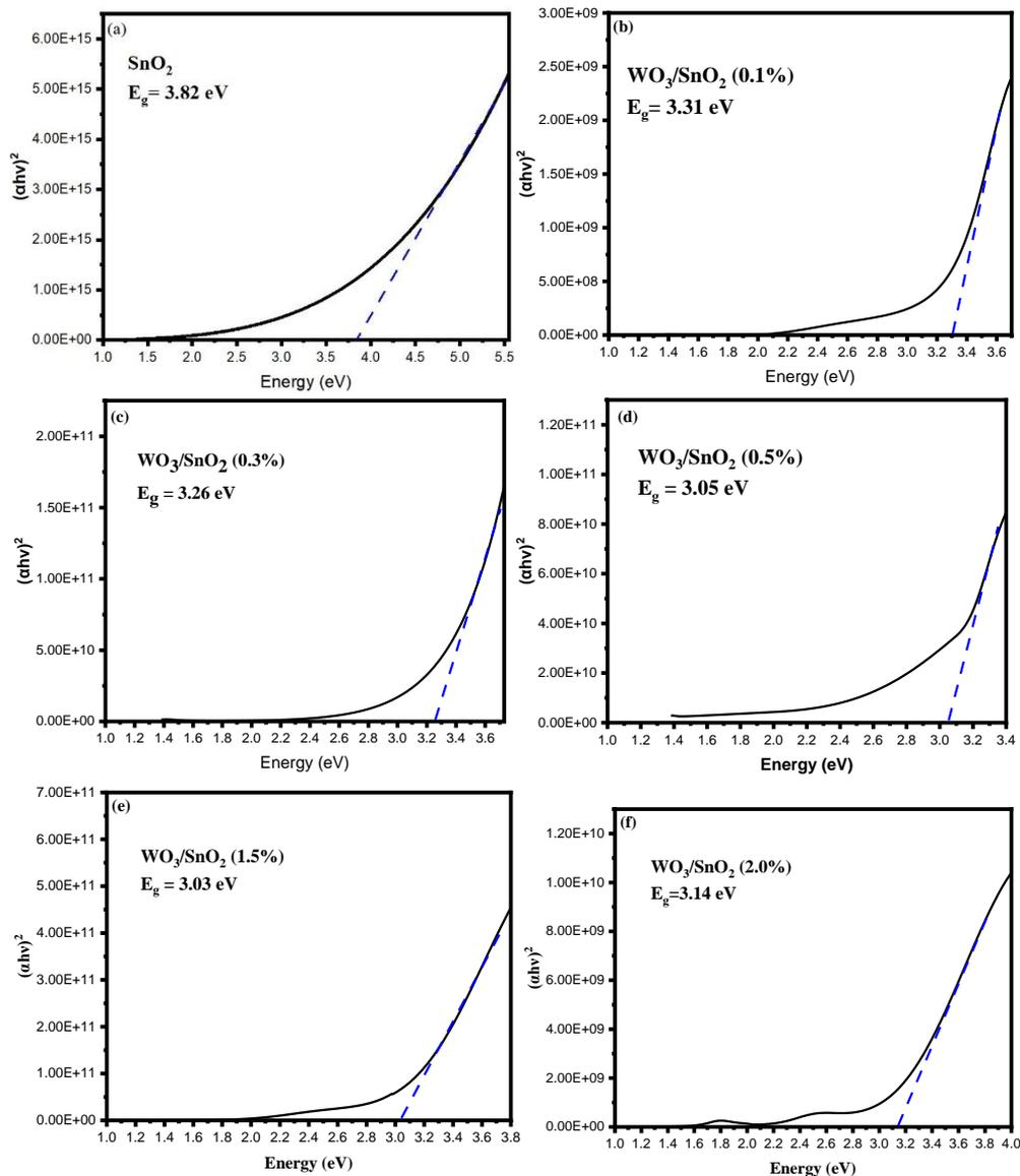
**Figure 4:** Plots of  $(\alpha h\nu)^2$  versus photon energy ( $h\nu$ ) for (a) pure  $SnO_2$ , (b)  $WO_3/SnO_2$  (0.1%) (c)  $WO_3/SnO_2$  (0.3%), (d)  $WO_3/SnO_2$  (0.5%) (e)  $WO_3/SnO_2$  (1.5%) and (f)  $WO_3/SnO_2$  (2.0%) thin films.
