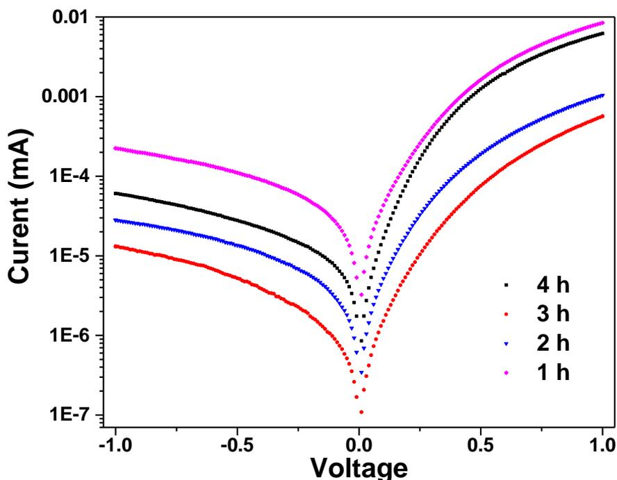
**Figure 6:** Semi logarithmic  $I$ - $V$  characteristics of FTO/ZnO/Au Schottky diode measured in the dark.
