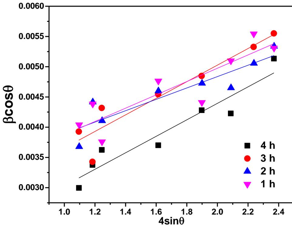
Figure 3: Williamson-Hall plot of ZnO nanorods prepared at different time intervals.
