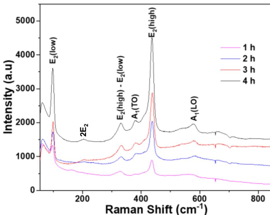
**Figure 5:** Room temperature Raman spectra of flower-like ZnO nanorods as a function of growth time.
