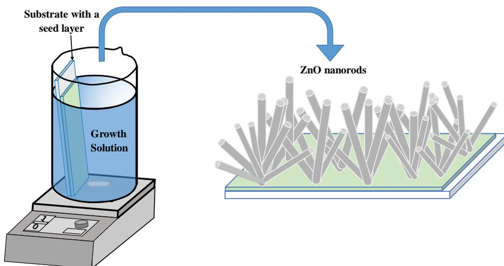
**Figure 1:** Schematic illustration of the setup for CBD employed in this study and ZnO nanorods.
