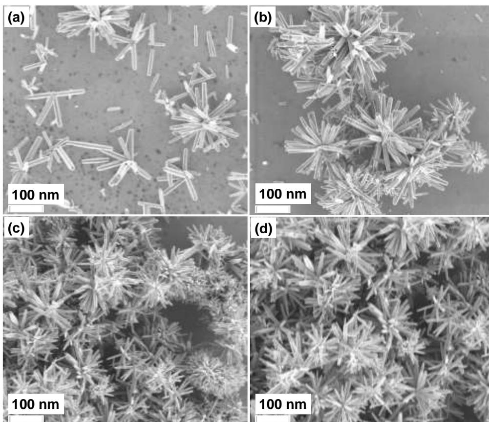
**Figure 4:** FESEM images of flower-like ZnO nanorods as a function of growth time: (a) 1 h, (b) 2 h, (c) 3 h and (d) 4 h
