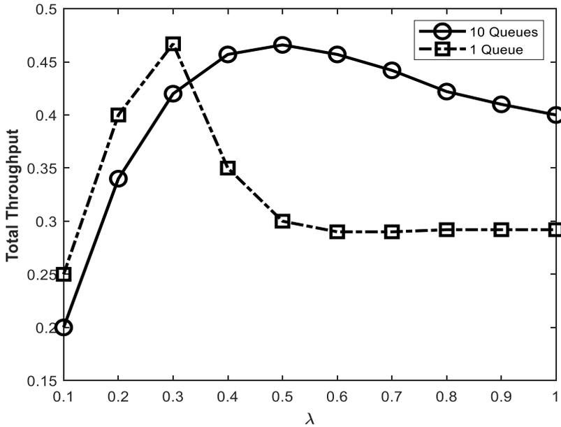
**Figure 8:** Variation of throughput with packet generation rate.
