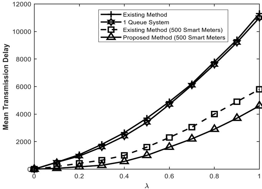
Figure 11: Mean transmission delay vs packet generation.
