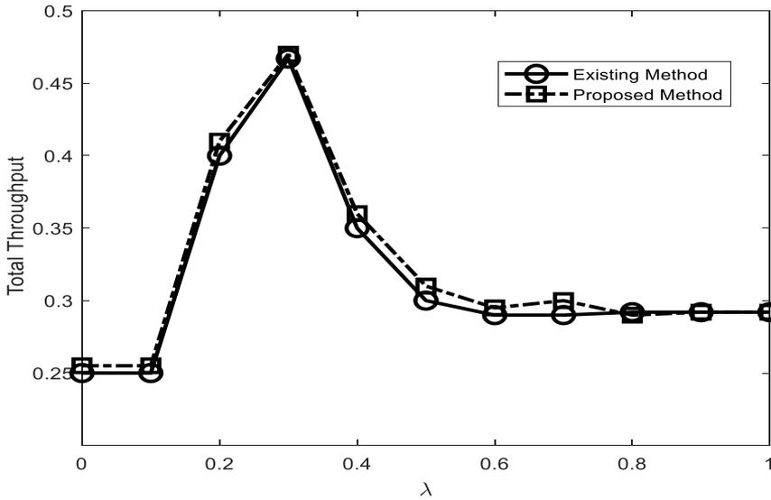
Figure 9: Variation of throughput with packet generation rate.
