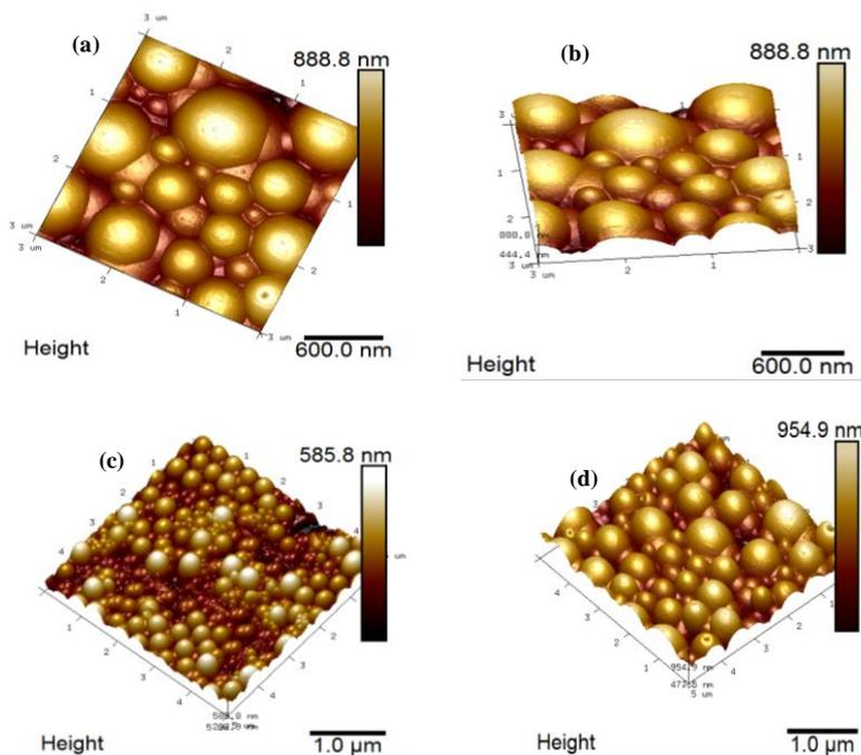
**Figure 5:** (a, b, c & d) Three dimensional (3D) images of P(St-MMA-AA) colloidal crystals viewed by atomic force microscope.
