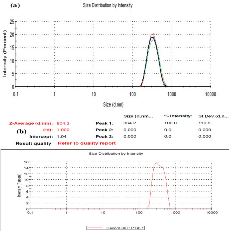
**Figure 2:** (a) size distribution intensity (b) dynamic light scattering graph.
