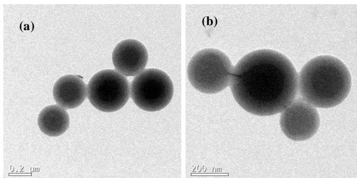
**Figure 4:** (a & b) Transmission electron micrographs of the synthesized P(St-MMA-AA) colloidal microspheres.
