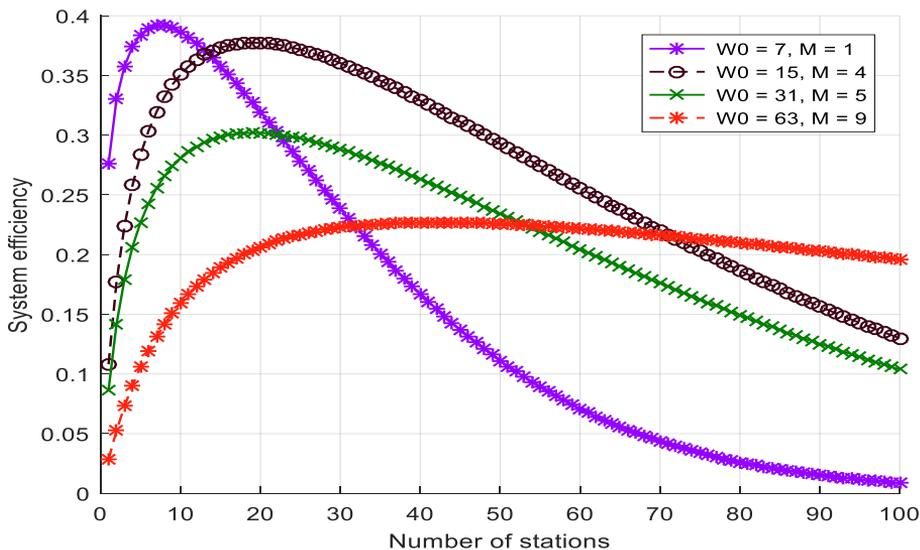
**Figure 5:** Relationship between system efficiency and the number of stations.
