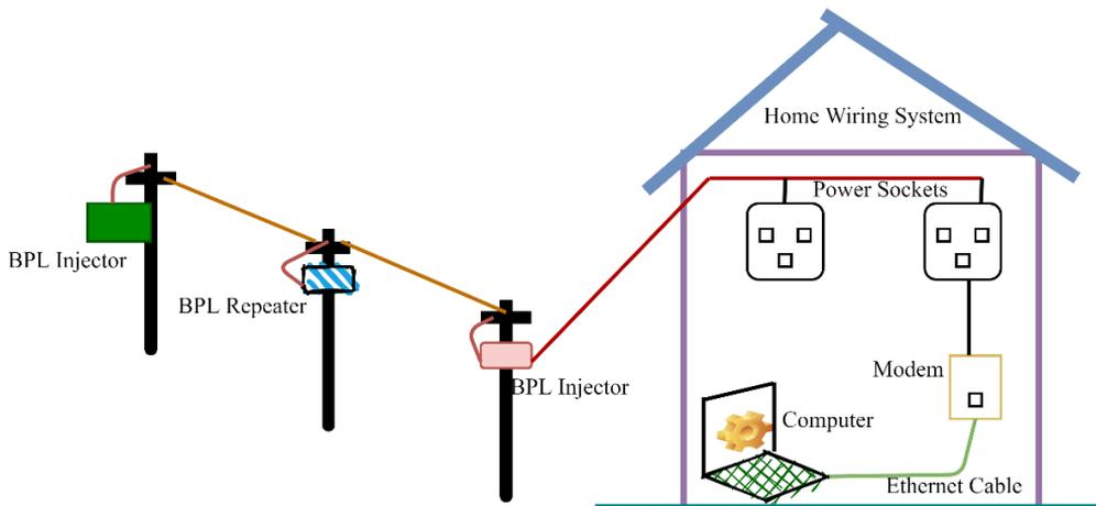
**Figure 1:** Power line communication technology.
