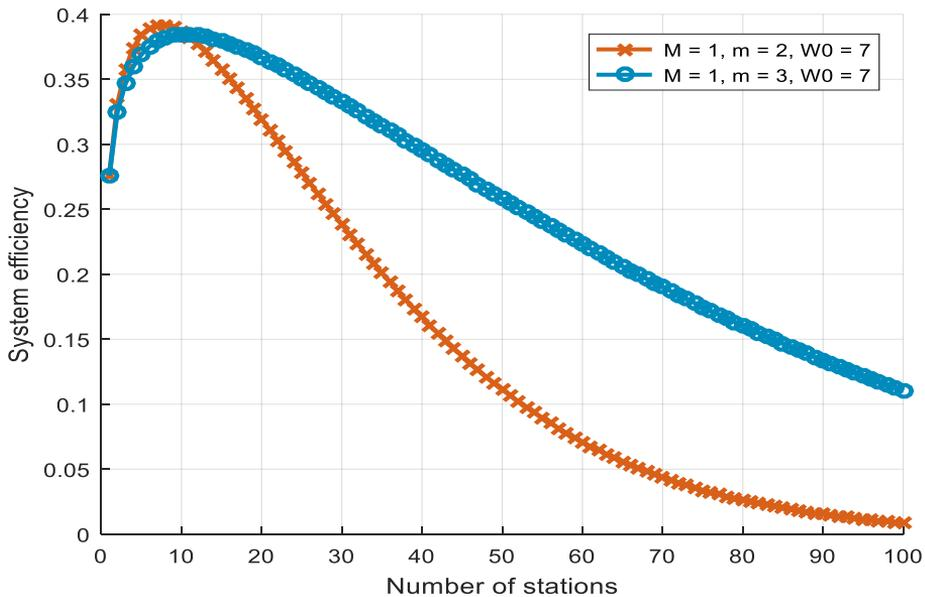
**Figure 4:** Relationship between system efficiency and number of stations.
