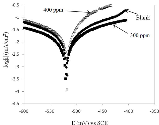
**Figure 1:** Polarization curves for mild steel electrodes in the absence and presence of 300 and 400 ppm *Acacia senegal* gum in 0.5 M  $H_2SO_4$  solutions (pH 0.7) at 35 °C.
