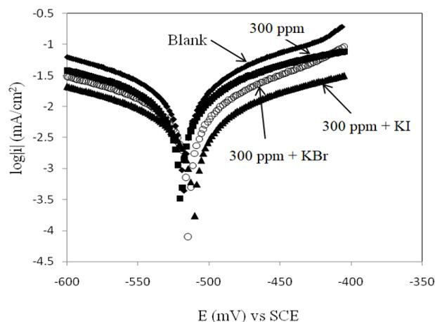
**Figure 3:** Polarization curves for mild steel electrodes in the presence of 300 ppm *Acacia senegal* gum + 0.08 M halide ions (KBr and KI) at 35 °C.
