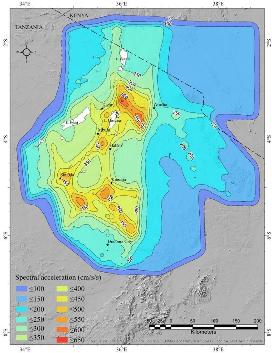
**Figure 7:** The ground shaking levels within the NTD at the spectral ordinate of 0.2 sec represented as spectral acceleration (cm/s/s), 5% damping and for 475 years return period (Contour interval: 50 cm/s/s).
