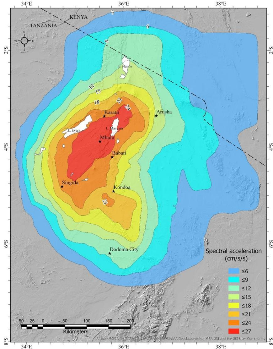
**Figure 8:** The ground-shaking levels within the NTD at the spectral ordinate of 2 seconds represented as spectral acceleration (cm/s/s), 5% damping, and for 475 years return period (Contour interval: 3 cm/s/s).
