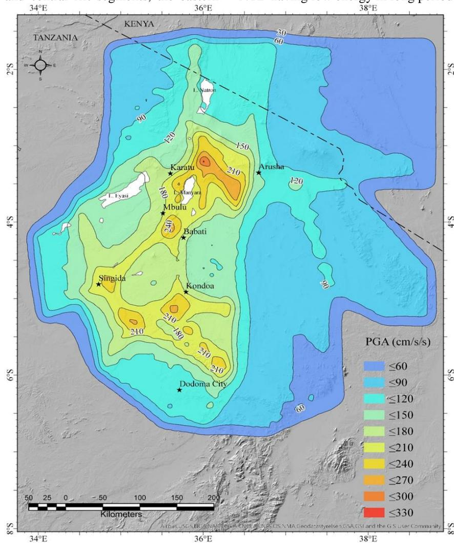
**Figure 6:** The ground shaking levels within the NTD at the spectral ordinate of 0.0 sec represented as PGA (cm/s/s), 5% damping and for 475 years return period (Contour interval: 30 cm/s/s).
