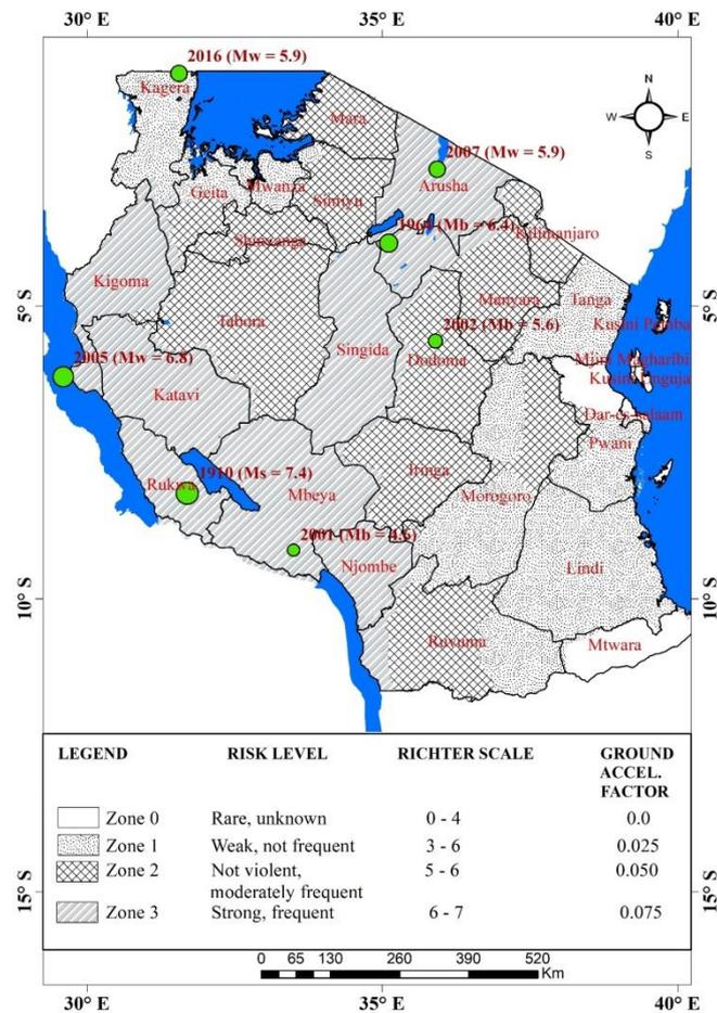
**Figure 1:** Earthquake Distribution for construction building code in Tanzania (Modified after NHBRU Technical Guideline No. 2 (Second Edition)). Green dots indicate damaging earthquake events recorded in Tanzania.
