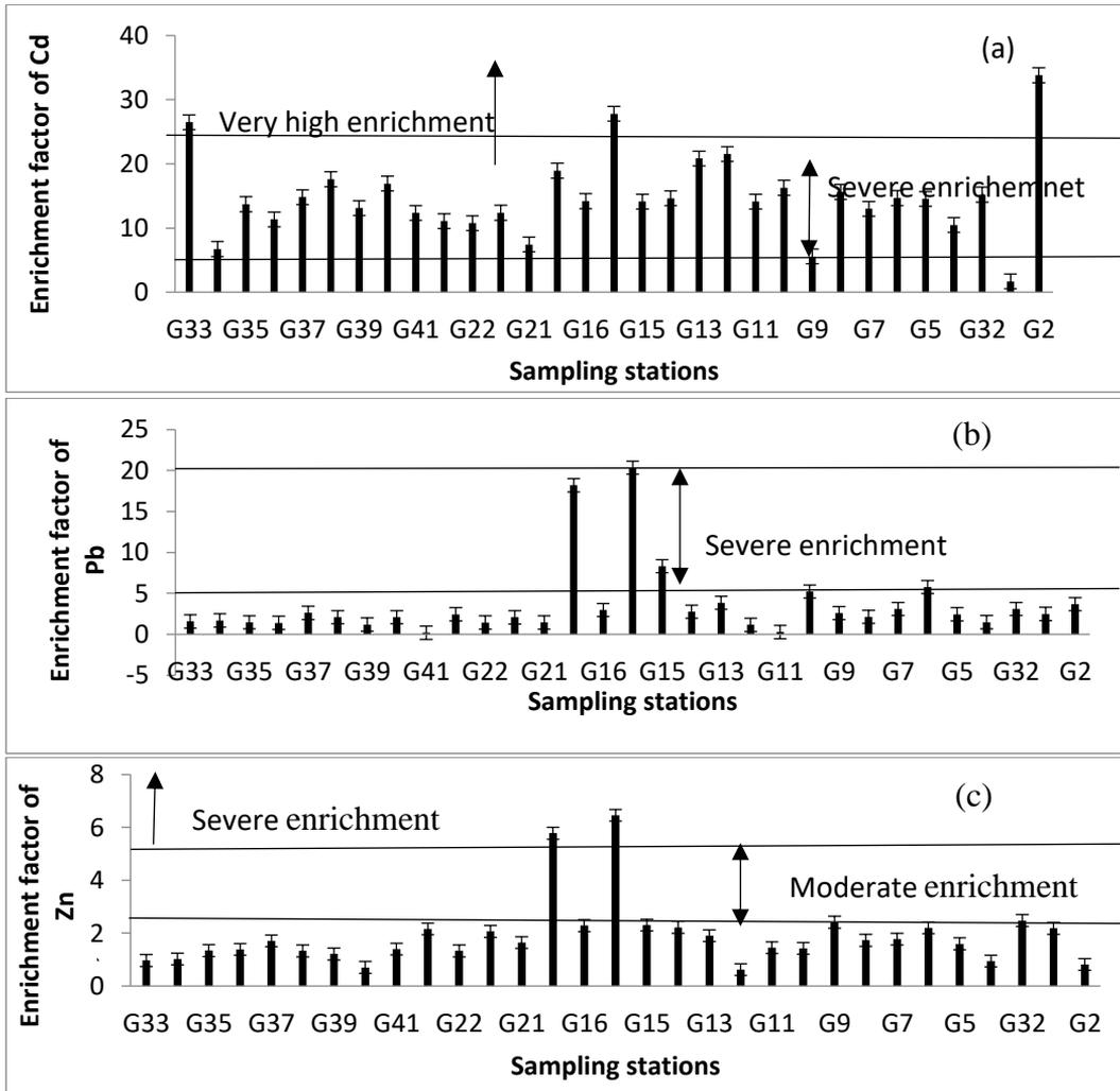
**Figure 3:** Three heavy metals of high enrichments in sediments along Dar es Salaam harbour channel.
