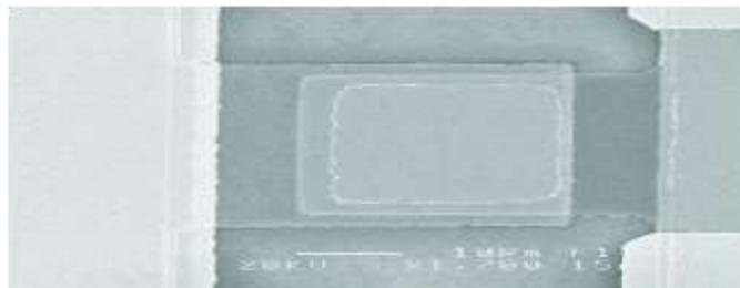
**Figure 2:** An SEM micrograph of one of the MgB<sub>2</sub>/Pd/Nb trilayer junctions fabricated.
