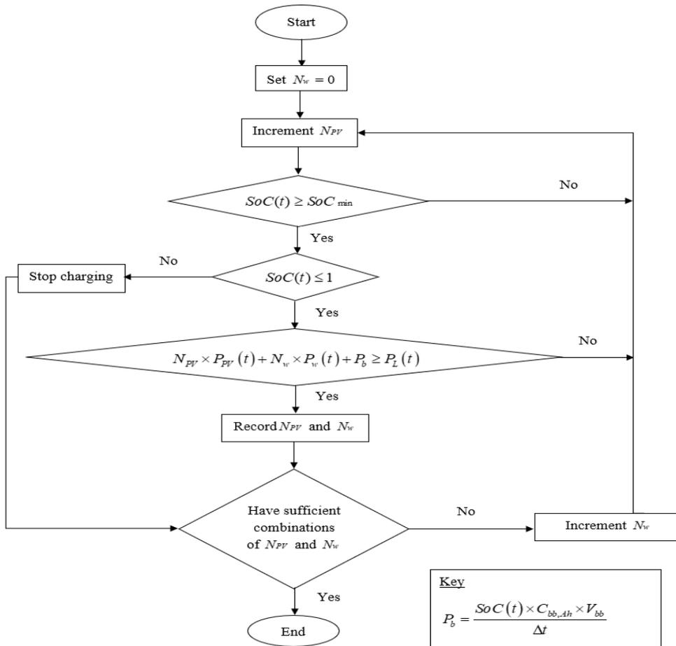
Figure 1: Wind and solar PV generations sizing flowchart.
