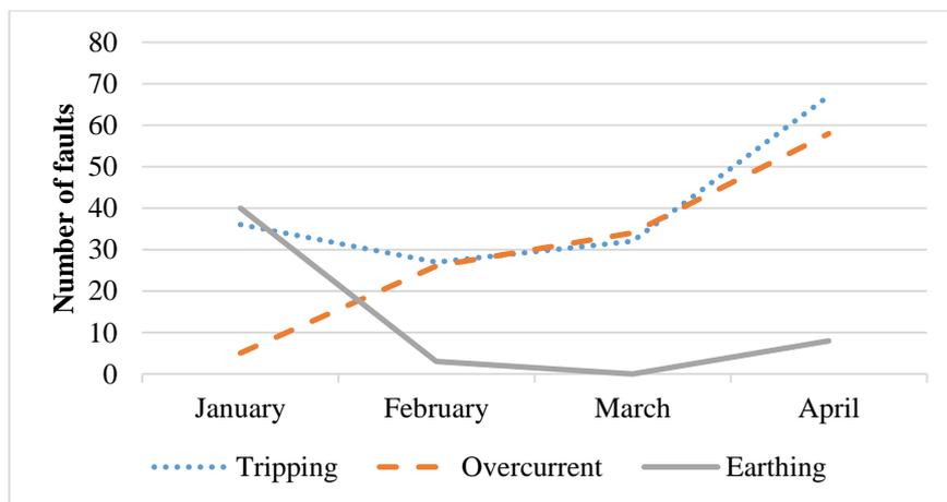
**Figure 1:** Sample stress faults statistics recorded from January–April 2018 at Ilala Substation (Source: TANESCO).
