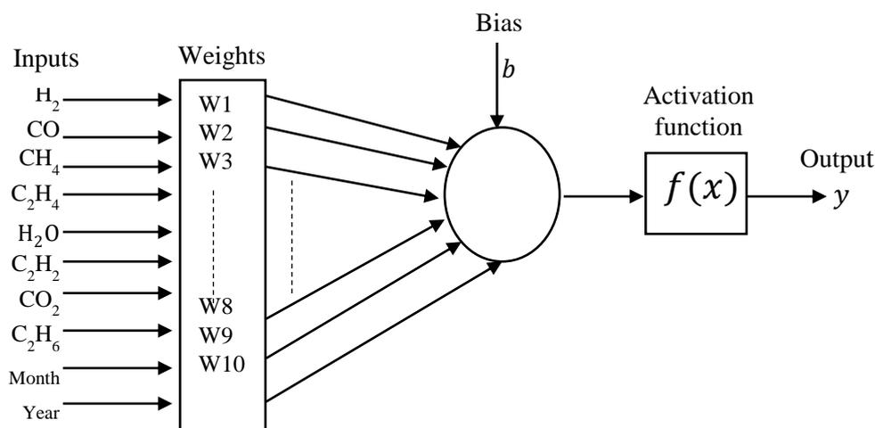
Figure 5: Structure of MLANN state prediction based on DGA data.
