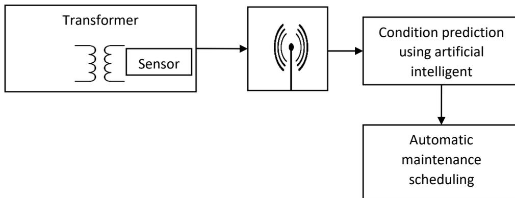
**Figure 3:** Proposed system architecture for transformer fault prediction in Tanzania secondary distribution network.
