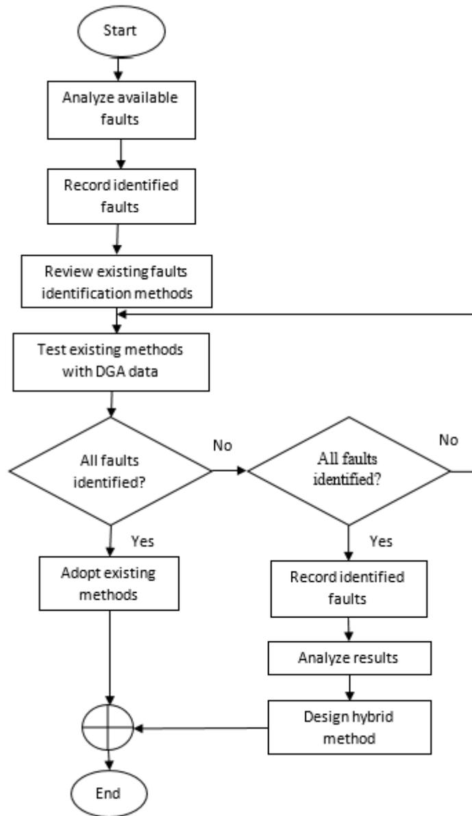
**Figure 6:** Fault identification method selection steps based on DGA.
