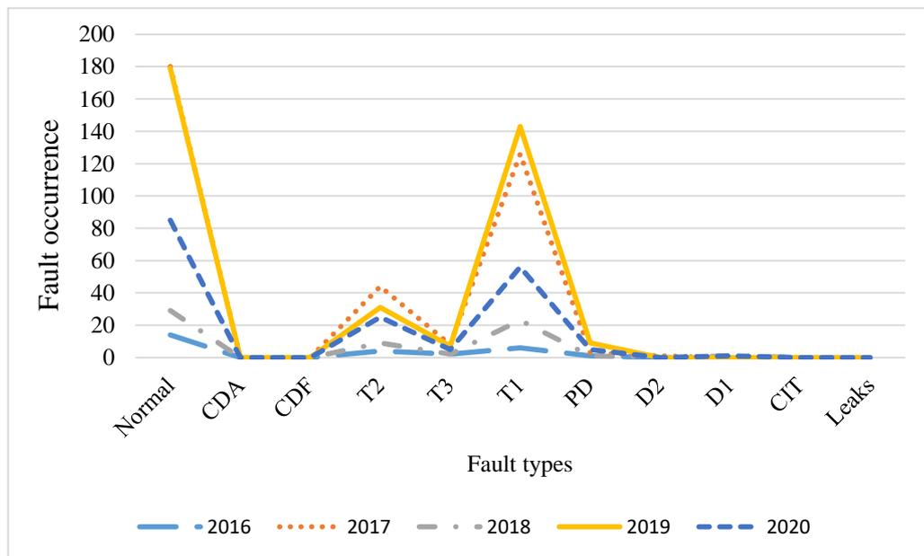
Figure 7: Faults identified by IEC 60599 method.
