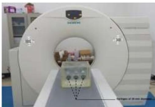
**Figure 1:** Typical irradiation set up of the phantom.
