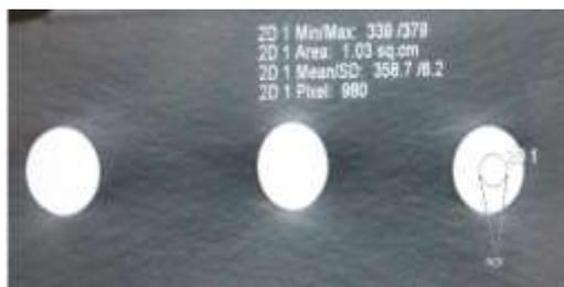
**Figure 2:** A cross sectional CT image of contrast phantom containing three syringes of 65 mL in volume that have been filled with different concentrations of iodinated of 300, 350 and 370 mg of iodine/mL CM.
