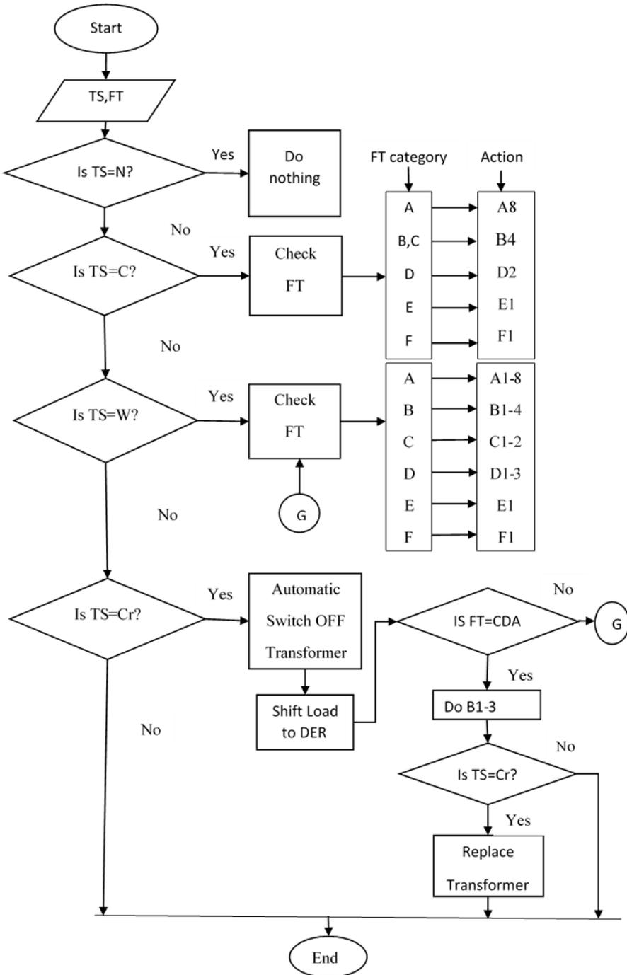
Figure 5: Decision-making process of the proposed KBS.
