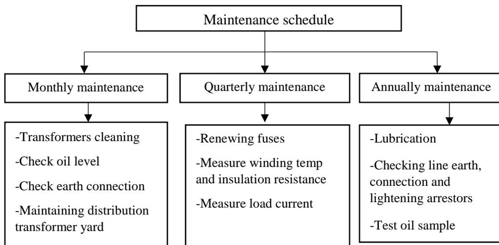
**Figure 1:** TANESCO transformer maintenance scheduling process.
