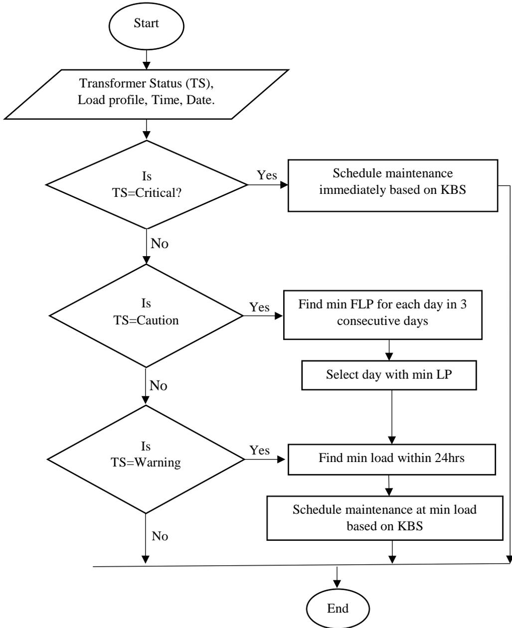
Figure 6: The FOTM design process.
