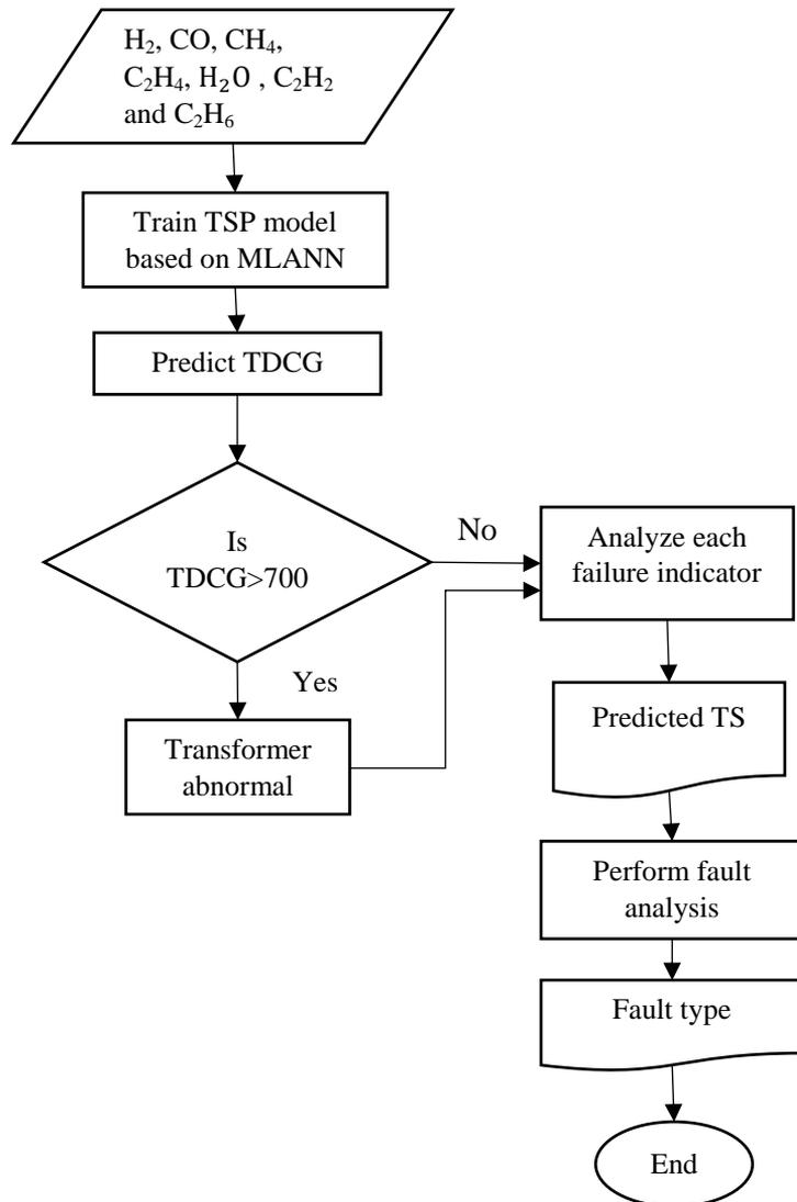
**Figure 4:** The architecture of the proposed TSP model.
