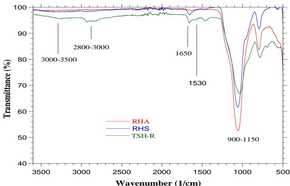
**Figure 3:** ATR-IR spectrum for RHA, RHS and TSH-R superimposed
