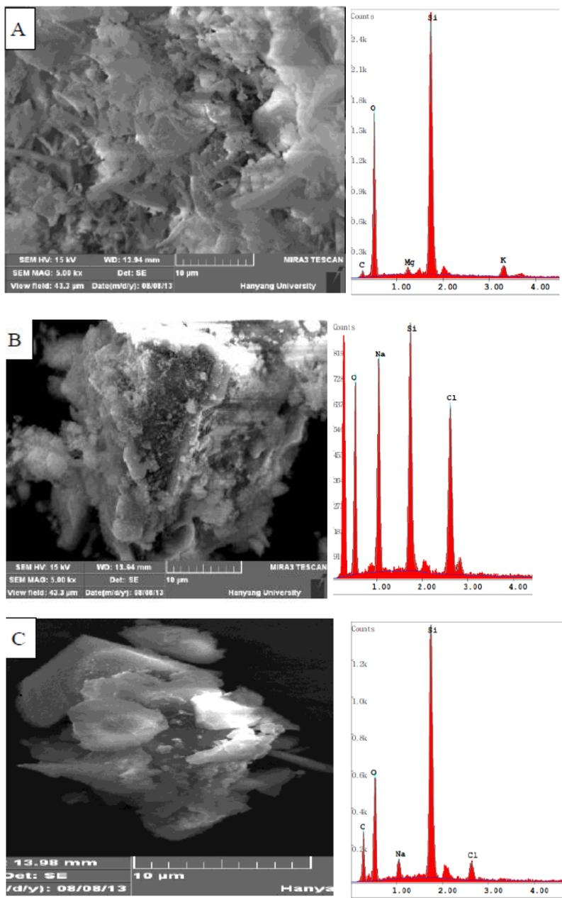
**Figure 5:** SEM micrographs and EDX spectra for A) RH, B) RHS and C) TSH-R
