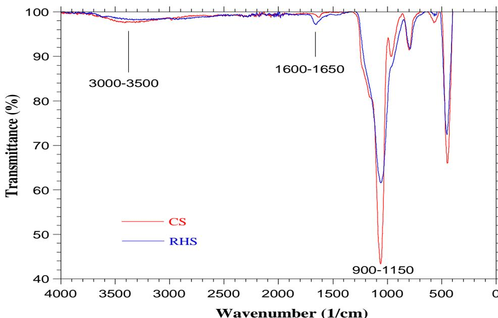
**Figure 2:** ATR-IR spectra for commercial silica (CS) and RHS.
