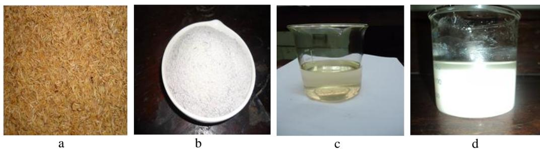
**Figure 1:** Pictures showing (a) raw rice husks (b) rice husks ash (c) Na<sub>2</sub>SiO<sub>3</sub> solution and (d) white silica precipitates.
