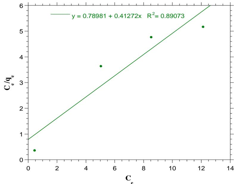
**Figure 7:** Langmuir adsorption isotherm for lead (II) ions on TSH-R
