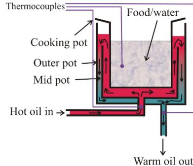
Figure 1: The schematic design of: A) the 3-tank TES system B) the mechanical thermostat and C) the cooking unit.
