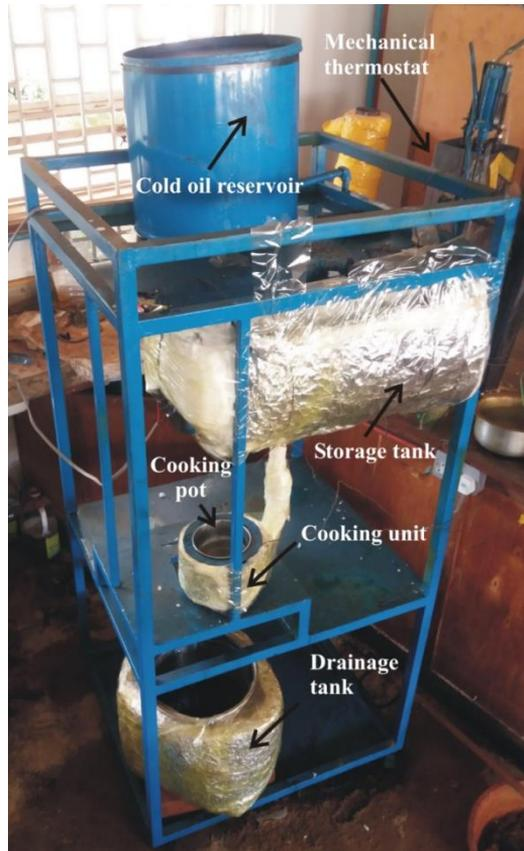
**Figure 2:** The photograph of the experimental setup for the 3-tank TES system.
