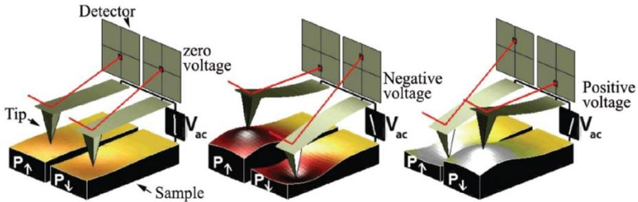
**Figure 3:** Schematic of PFM operation. The sample deforms in response to the applied voltage. The resulting cantilever deflection is detected and interpreted in terms of the domain patterns of the sample (Asylum Research 2022).
