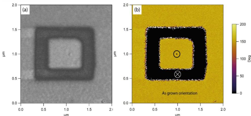
**Figure 8:** 30 nm thick PZT 50/50 with 15% excess PbO on SRO. (a) AFM (a) PFM Vertical amplitude and (c) PFM Vertical phase. As-grown thin film has an upward polarization direction. The switched bottom region was obtained by poling the sample with +5V dc bias on the AFM tip.
