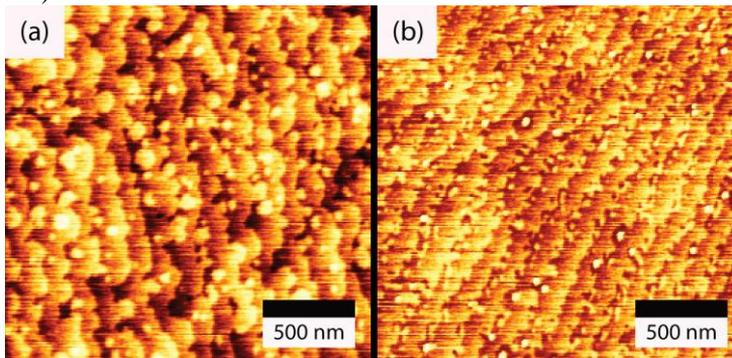
**Figure 7:** AFM image of (a) 2 nm SRO and (b) 30 nm PZT 50/50 thin films. The roughness of PZT and SRO are about 0.144 nm and 0.149 nm, respectively.
