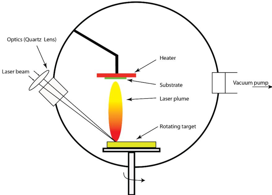
**Figure 2:** Schematic diagram of a PLD system.
