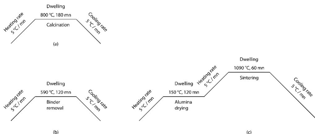
**Figure 1:** Heat treatment profiles and parameters for calcination and sintering parameters. (a) Calcination, (b) Binder removal step before final sintering, and (c) Two-step sintering: the first step involves drying of alumina paste used to seal crucibles to minimize PbO loss and the second step is the high-temperature sintering.
