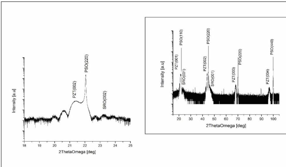
**Figure 6:** 2theta-Omega patterns for (002) peak of PZT 50/50 and SRO, and full scan pattern (insert).
