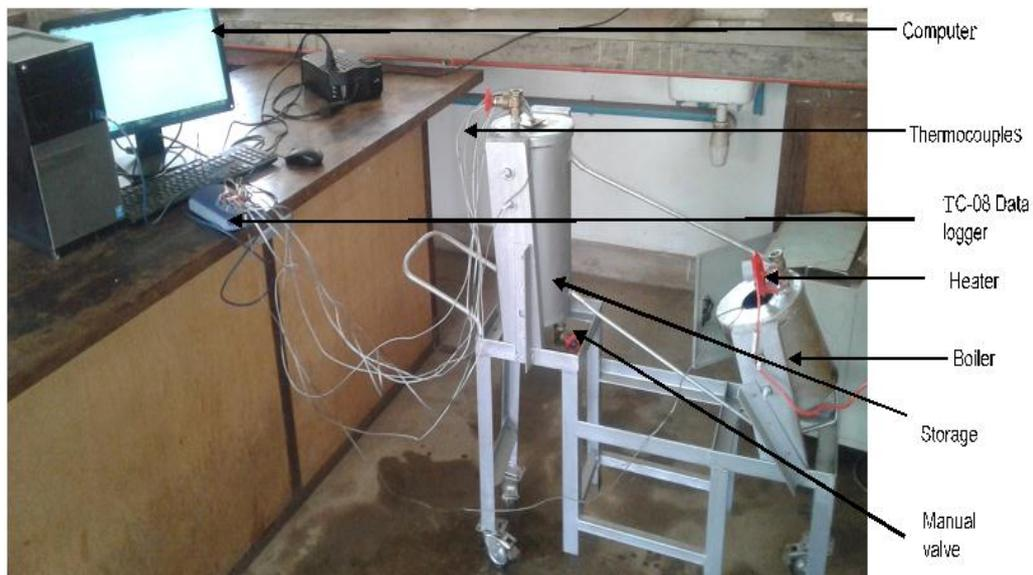
**Figure 4:** The experimental setup showing charging of the storage tank by thermosiphon principle in which eight thermocouples were connected to a TC-08 data logger to monitor the tanks' temperatures.
