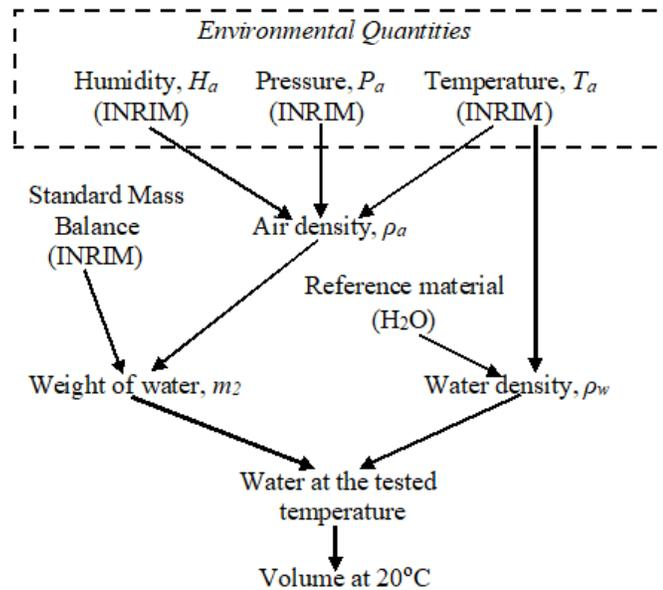
Figure 7: Traceability of uncertainty chain for volume measurements at INRIM (Lorefice 2009).
