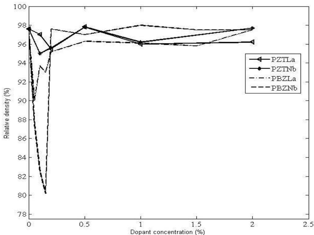
**Figure 2:** Relative density as function of dopants concentrations.
