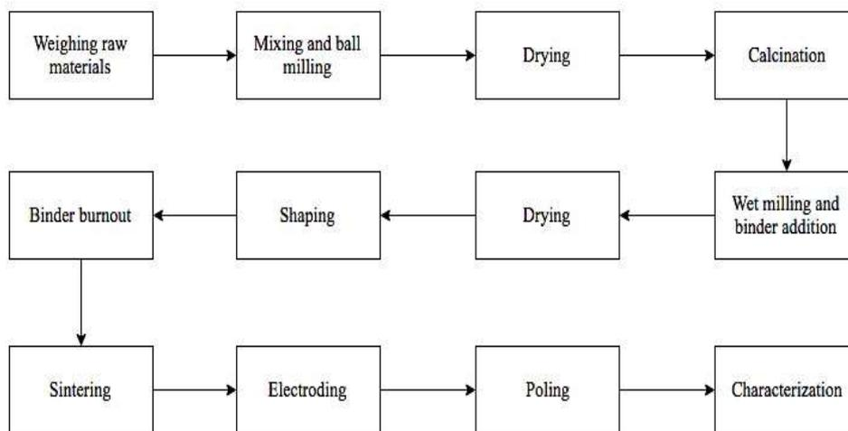
**Figure 1:** The flow chart showing the steps of the processing of PZT and PBZ (Richerson 2006).
