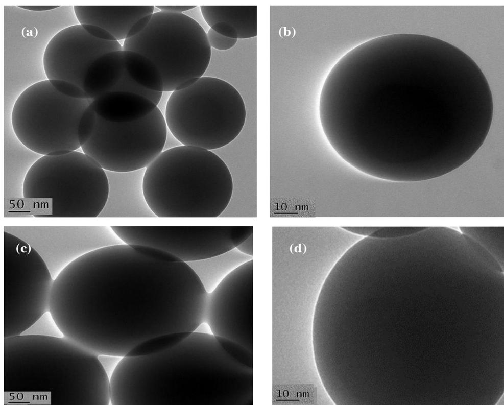
**Figure 2:** Transmission electron micrographs of (a) 200 nm (b) 130 nm (c) 295 nm (d) 158 nm as-synthesized P(St-MMA-AA) microspheres.
