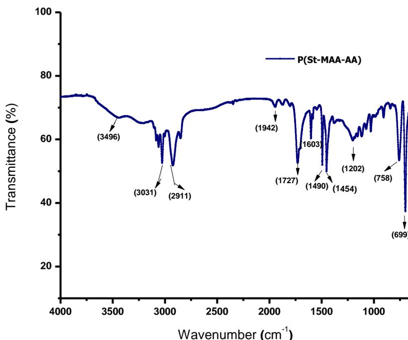
**Figure 1:** Fourier transform infrared (FTIR) spectrum of the as-synthesized P(St-MMA-AA) latex.
