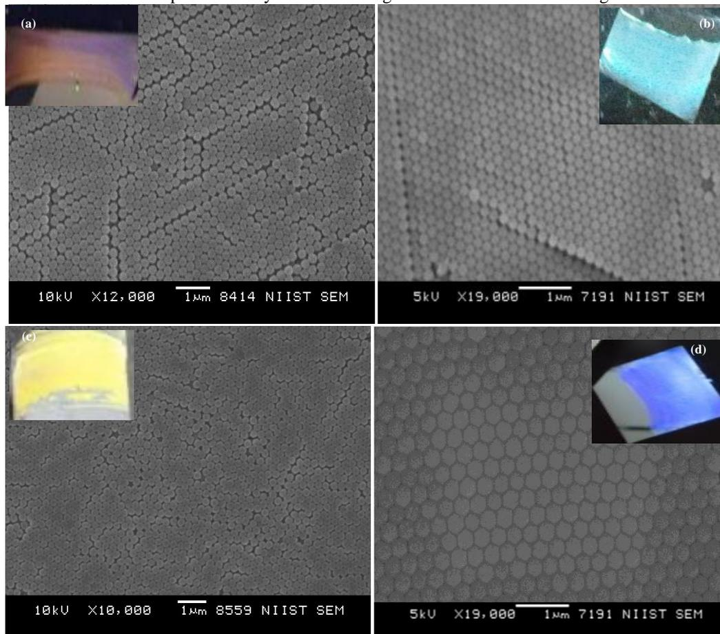
**Figure 3** (a, b, c and d): Scanning electron micrographs of the fabricated photonic crystal films with insets of the obtained photonic crystal films on glass slides.
