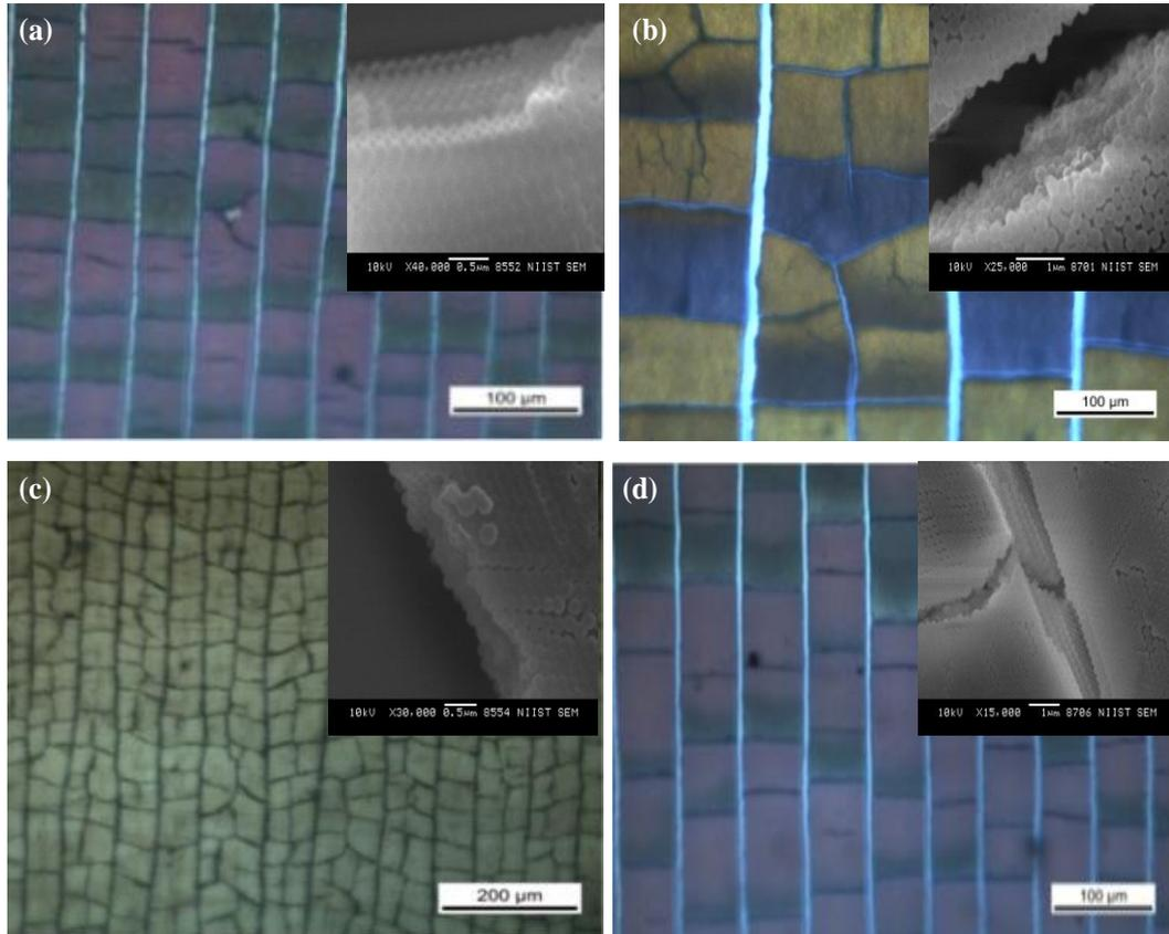
**Figure 4:** Optical electron micrographs with insets of scanning electron micrographs of the fabricated photonic crystals.
