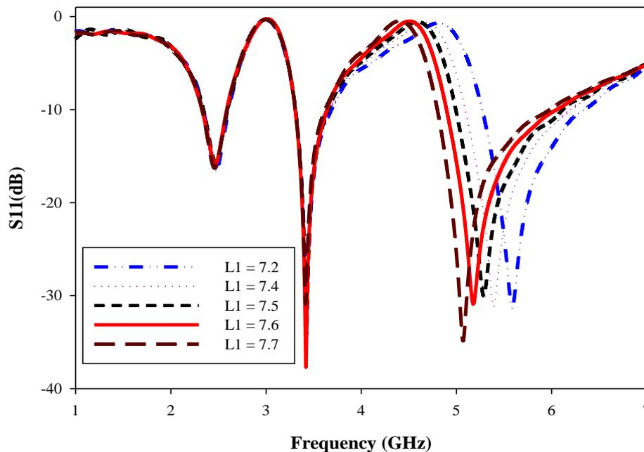
**Figure 3:** Effect of return loss results with the variation of length  $L_1$ .
