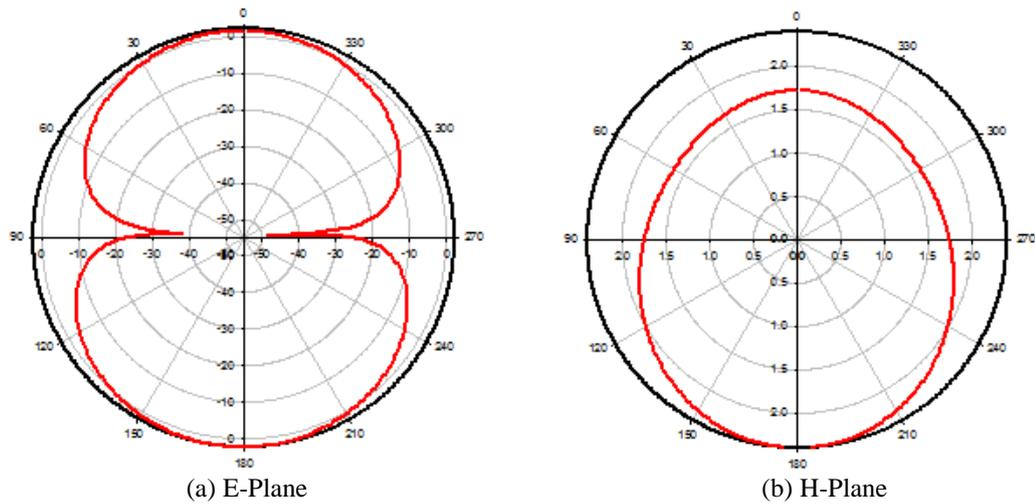
**Figure 13:** Simulated radiation patterns at 3.5 GHz.
