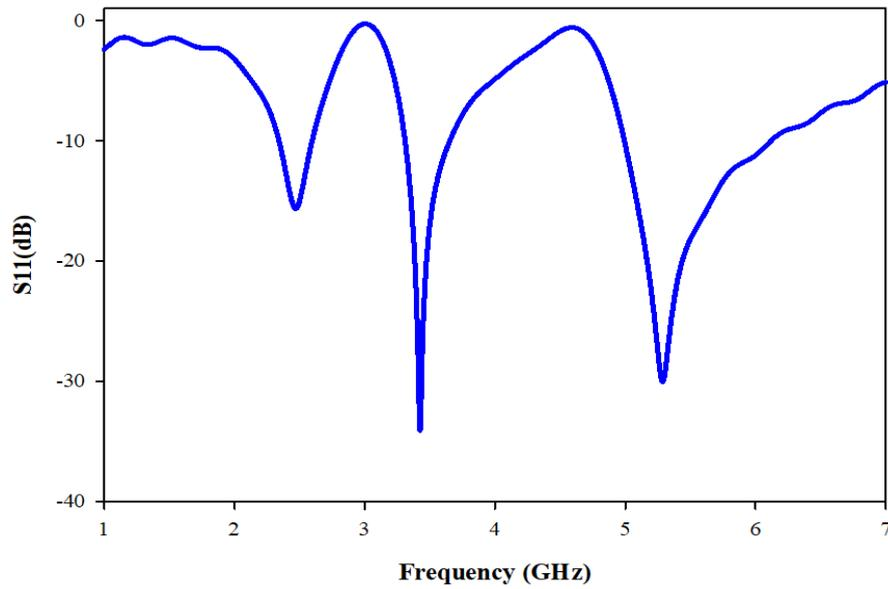
**Figure 11:** Simulated return loss results of the proposed multi-band antenna.
