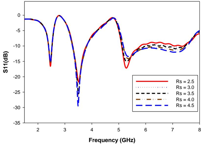
**Figure 8:** Effect of return loss results with the variation of ground slot length  $R_s$ .
