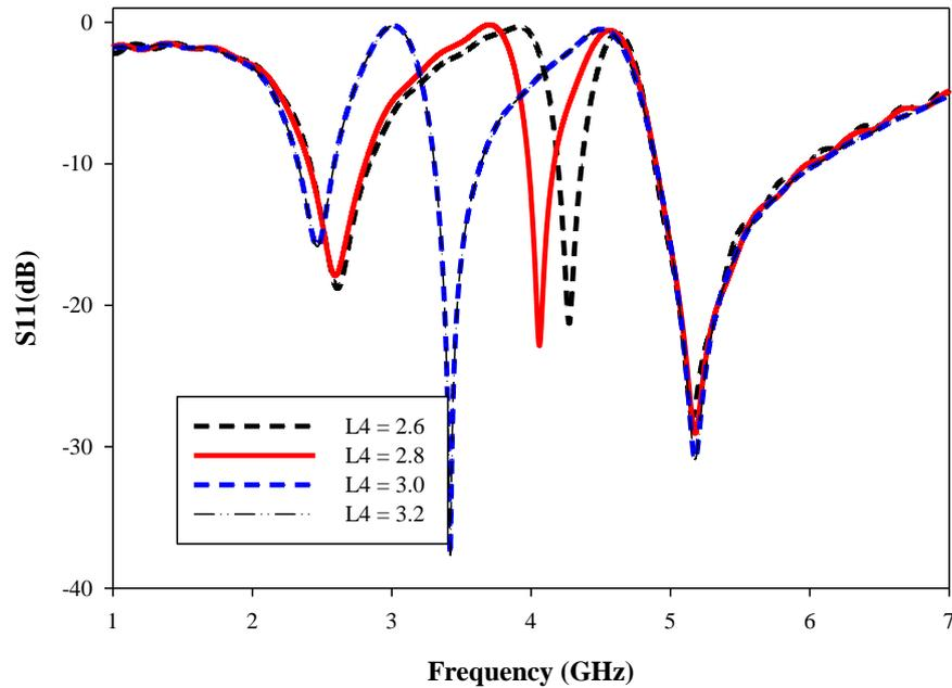
**Figure 5:** Effect of return loss results with the variation of length  $L_4$ .
