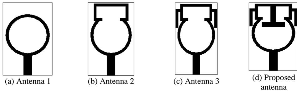
**Figure 1:** The geometry of the design process of multi-bands monopole antenna.
