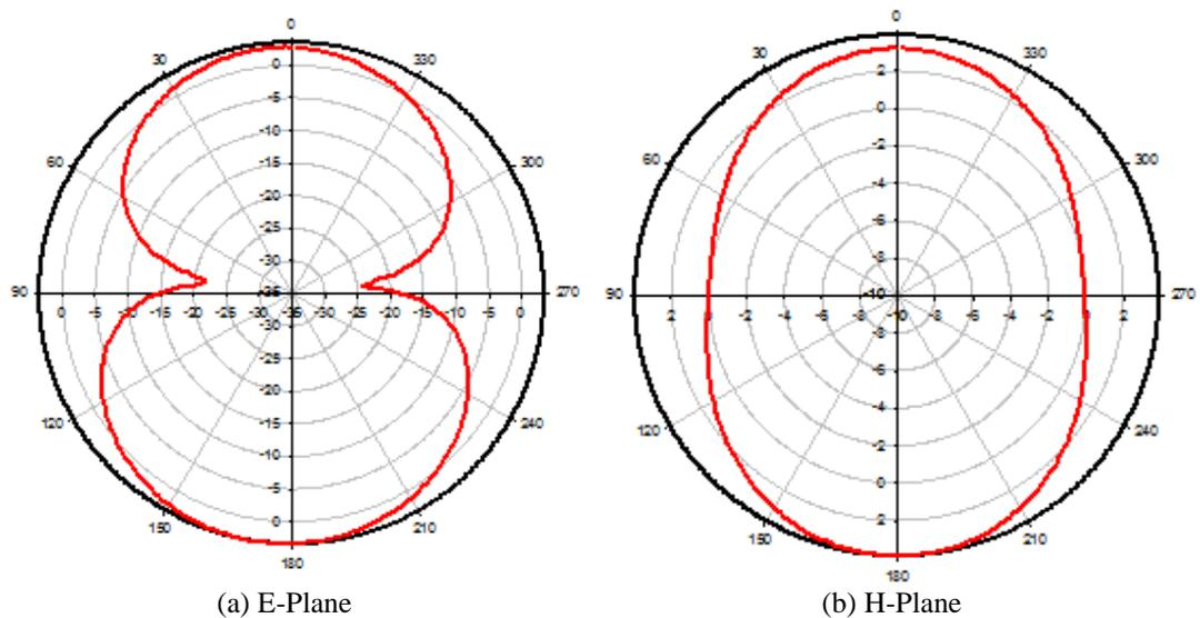
**Figure 14:** Simulated radiation patterns at 5.5 GHz.
