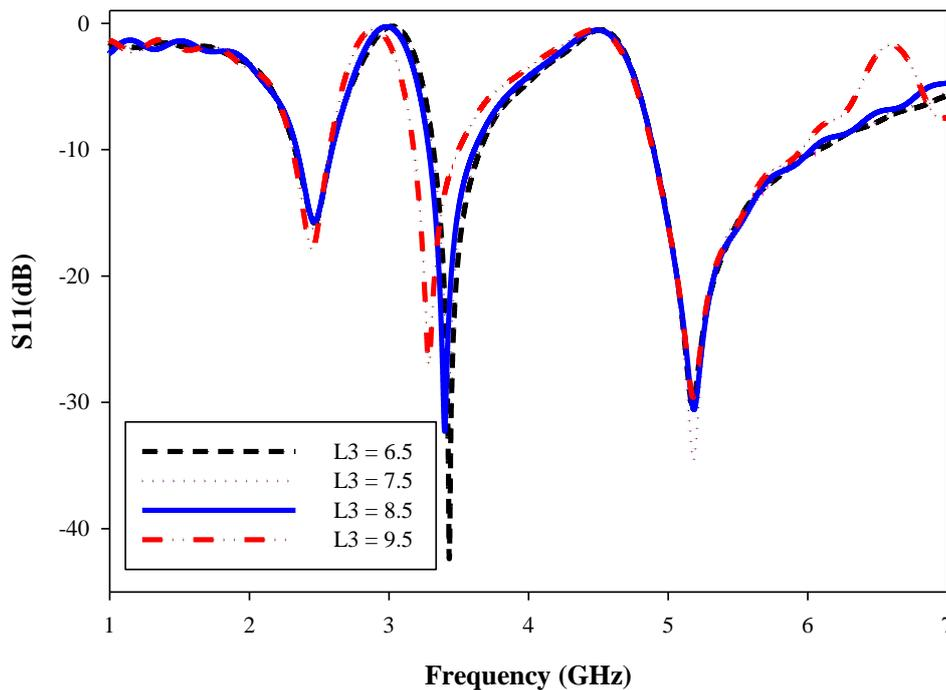
**Figure 4:** Effect of return loss results with the variation of length  $L_3$ .
