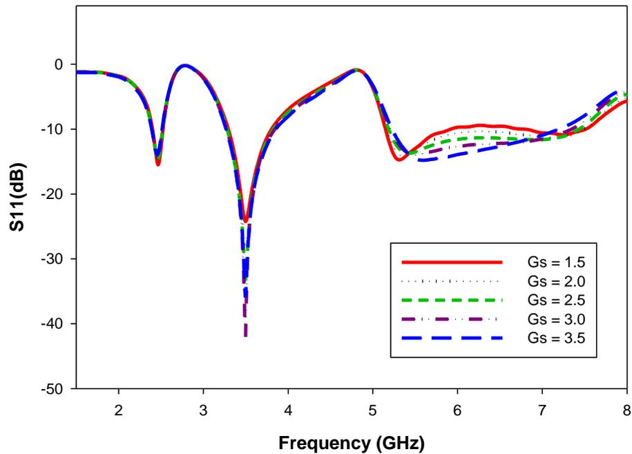
**Figure 7:** Effect of return loss results with the variation of ground slot width  $G_s$
