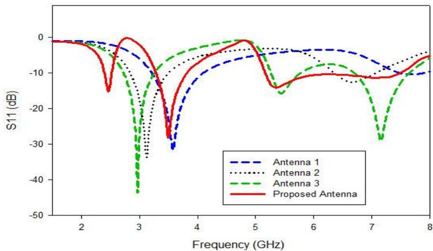
**Figure 2:** Simulated return loss of the proposed antenna.
