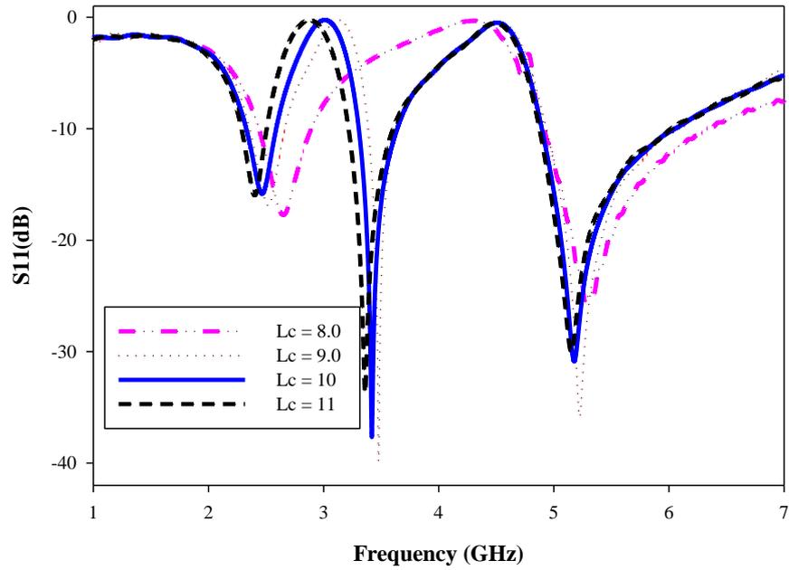
**Figure 6:** Effect of return loss results with the variation of length  $L_C$ .
