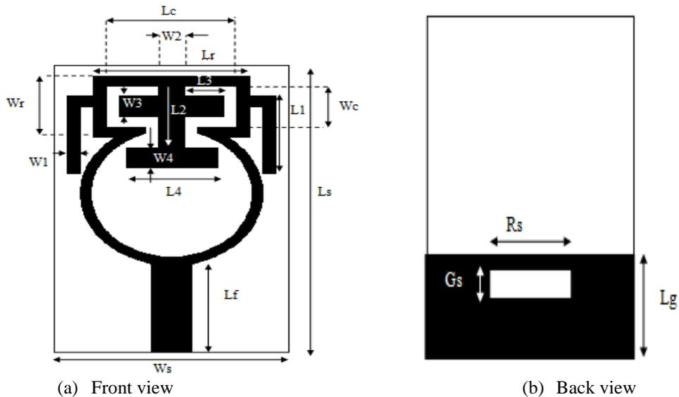
**Figure 9:** The Geometry of proposed multi-bands antenna.
