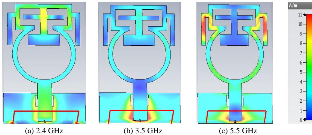
**Figure 10:** Surface current distribution of the proposed multi-bands antenna at (a) 2.4 GHz, (b) 3.5 GHz, and (c) 5.5 GHz.
