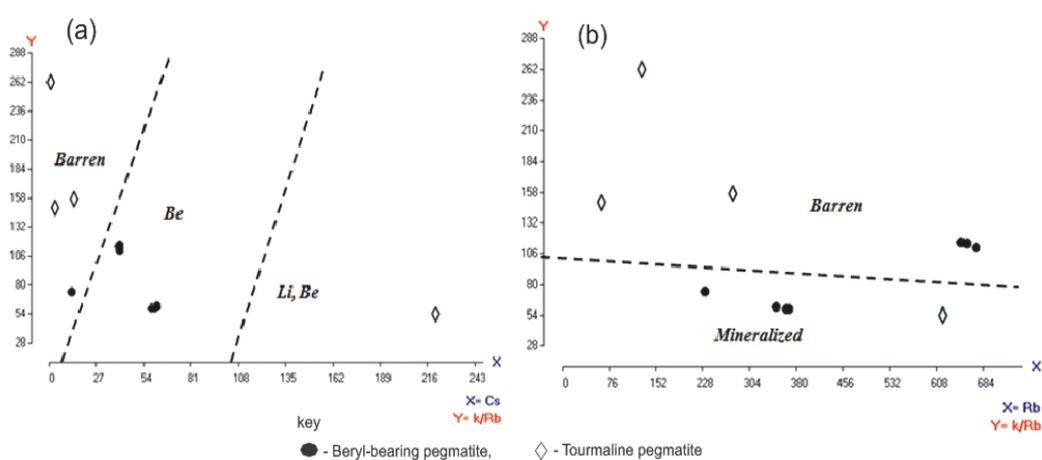
**Figure 7:** Discrimination diagrams showing the degree of fractionation and mineralisation of Olode pegmatites: (a) Cs vs K/Rb (Trueman and Cerny 1982), (b) Rb vs K/Rb (Stavrove et al. 1969).
