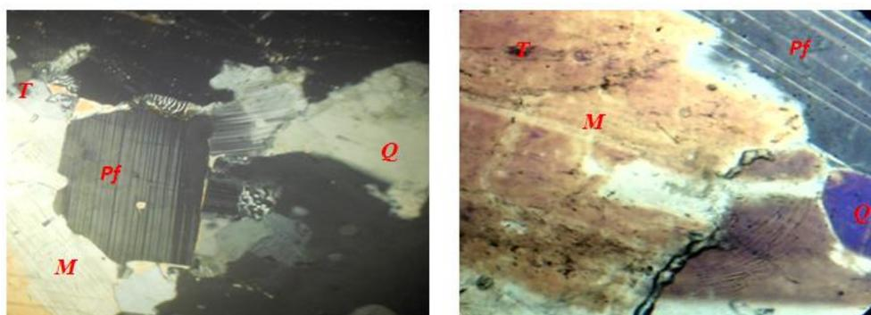
**Figure 3:** Photomicrographs of samples of tourmaline pegmatite from Olode study area under cross polarized light. Pf = Plagioclase feldspar, M = Microcline feldspar, Q = quartz (X40).
