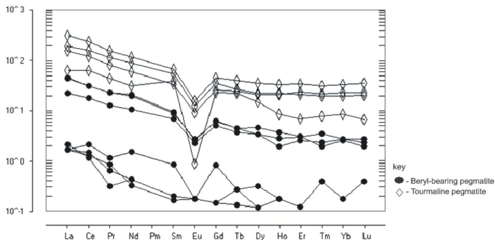
**Figure 6:** Chondrites-normalized REE patterns for the analysed pegmatites from Olode and environ.
