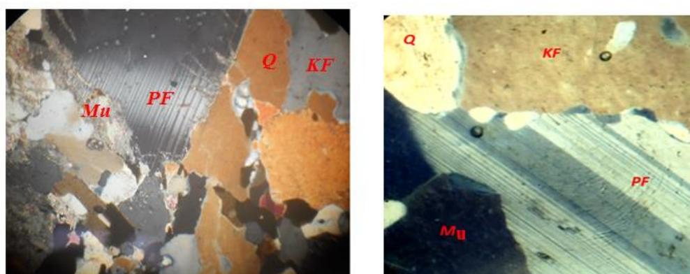
**Figure 4:** Photomicrographs of samples of the beryl-bearing pegmatite from Concord mines in Falansa under cross polarized light. PF = Plagioclase feldspar, KF = K-feldspar, Mu =Muscovite, Q = quartz (X40).
