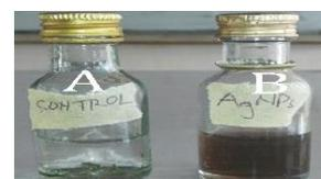
**Figure 2:** A, AgNO<sub>3</sub> as control; B, biosynthesized AgNPs after 30 minutes of bioreduction.
