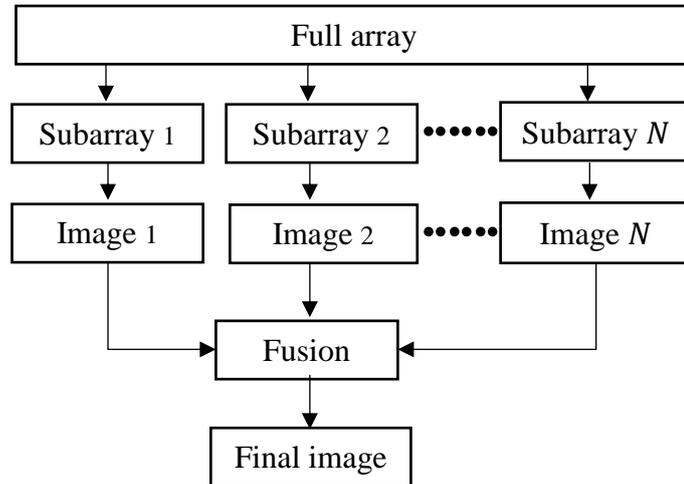
**Figure 2:** Multiple subarrays image formation.
