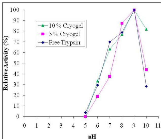
**Figure 6:** Effect of pH on Activity of Free trypsin and epoxy-MPAAGs Immobilized Trypsin
