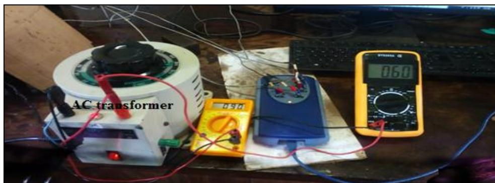
**Figure 8:** The speed control component of the system to vary the speed of the oil pump.
