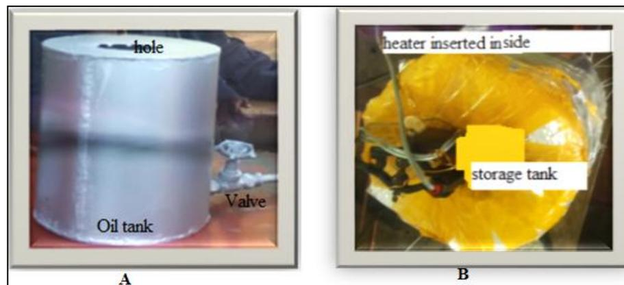
**Figure 5:** Hybrid TES tank constructed using mild steel material and coated with aluminium paint.
