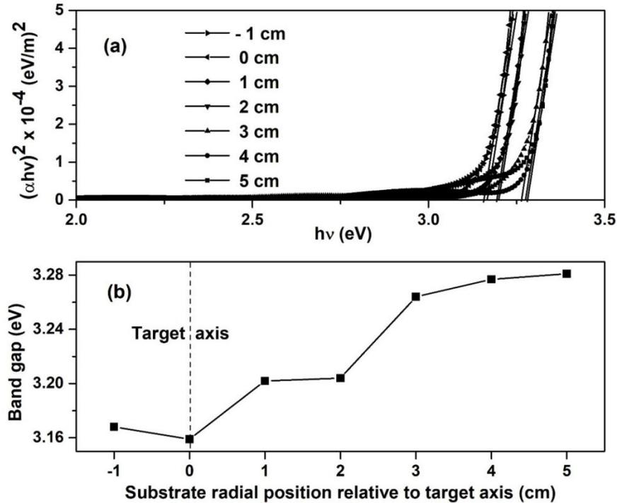
**Figure 6:** (a) Tauc's plot of  $(\alpha hv)^2$  versus  $h\nu$  (b) Optical band gap of ZnO thin films as a function of substrate radial position.
