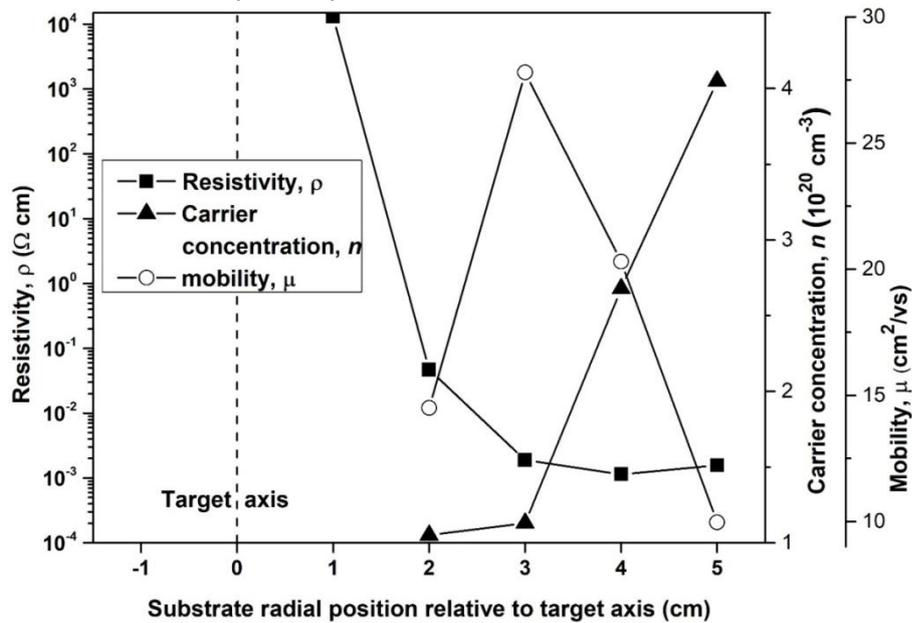
**Figure 4:** The variation of resistivity, carrier concentration and mobility of ZnO thin films with substrate radial position.
