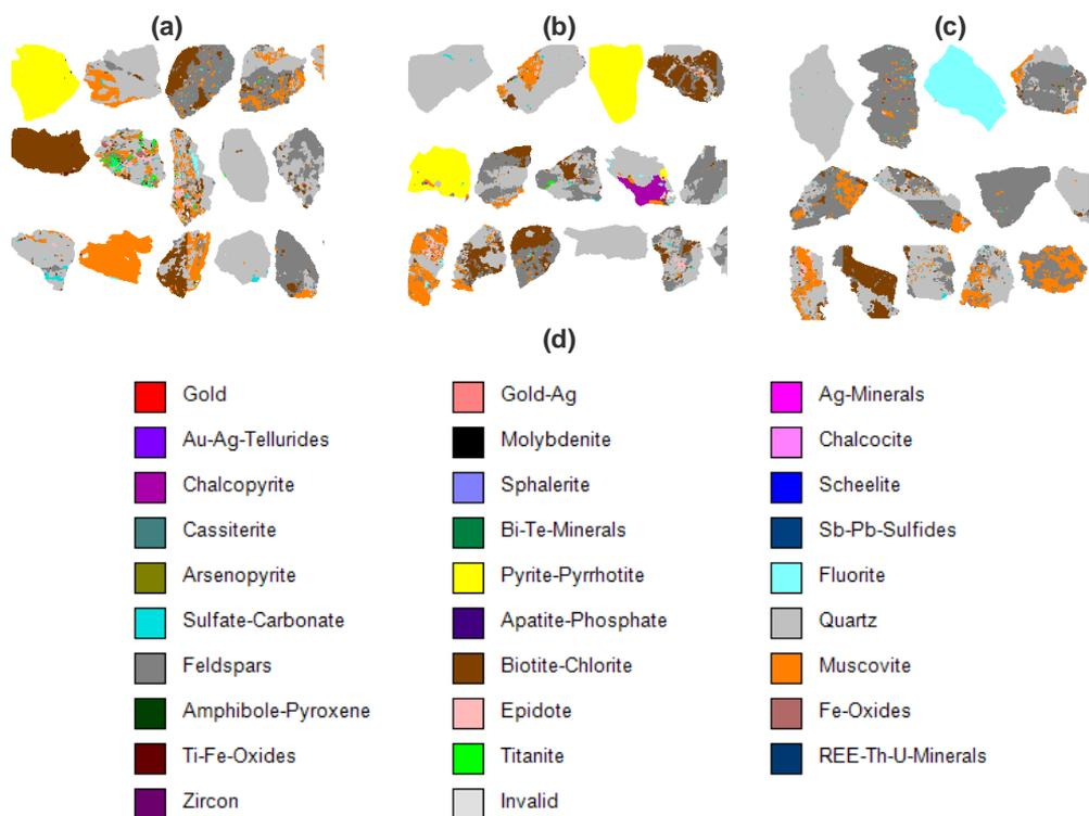
**Figure 5:** MLA particle shape images for Buzwagi ore comminution products: (a) Sample S1-6, (b) Sample S2-6, (c) Sample S3-6 and (d) Legend.
