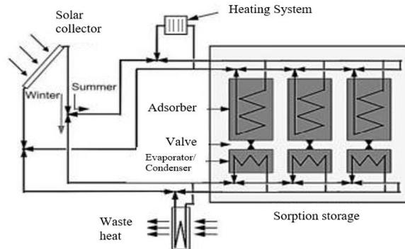
**Figure 4:** Seasonal adsorption thermal storage system, (Adapted from Hauer 2007).
