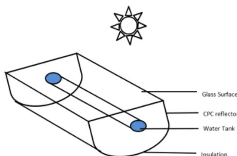
**Figure 7:** Cross-sectional schematic of the compound parabolic concentrating collector integrated with PCM, (Chaabane et al 2014).
