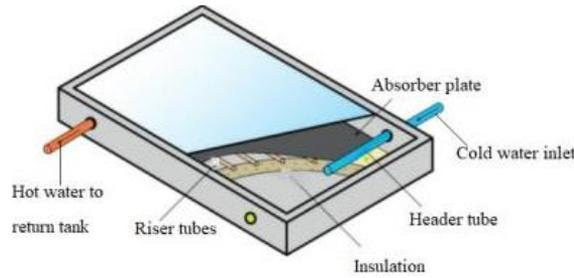
**Figure 1:** Absorber layer made of metallic tubes, (Adapted from Tripathi and Aijaz 2014).
