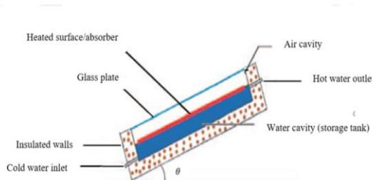
**Figure 14:** Cross-sectional representation of the SWH, (Bello and Odey 2009)
