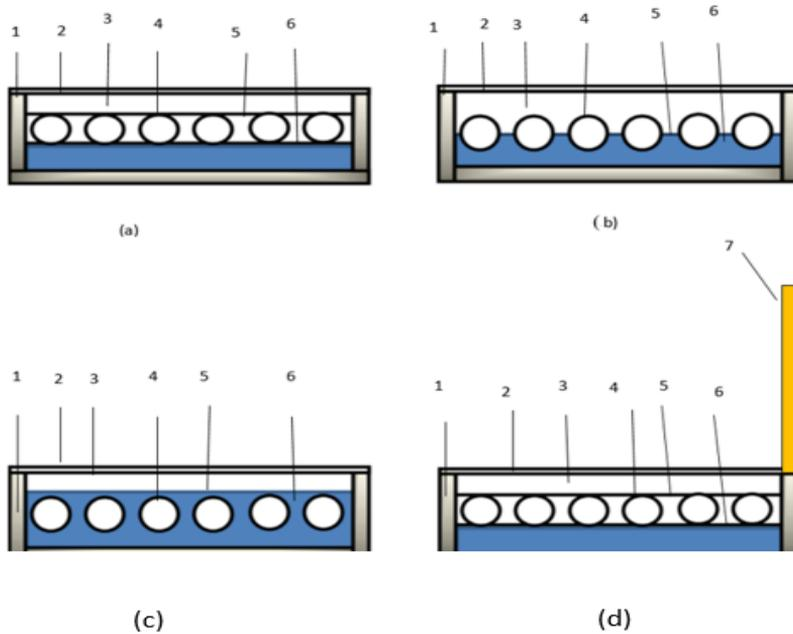
**Figure 6:** Schematic representation of a flat plate solar collector with TSF in thermal storage technologies, (Adapted from Faud and Kerswani, 1973) (a)below tubes, (b)half perimeters of the tubes, (c)immersed tubes, (d)with reflector, (1) insulation, (2) glass cover, (3) air space, (4) tubes, (5) absorber plate, (6) TSF, (7) reflector.
