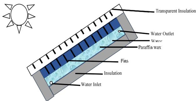
**Figure 6:** Integrated collector storage solar water heater with fins inside the wax, (Reddy 2007)
