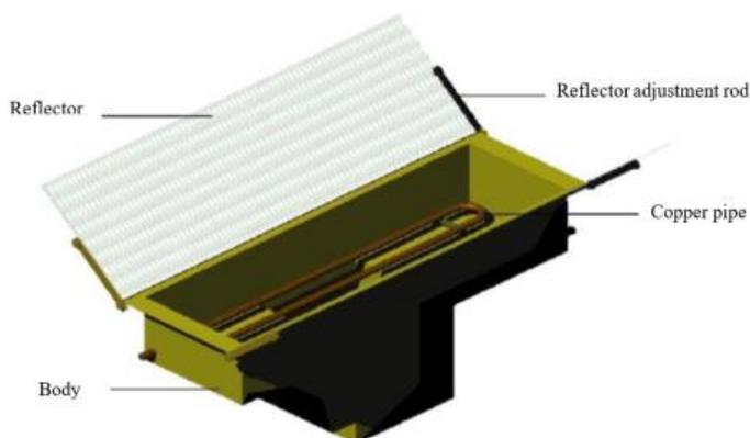
**Figure 9:** Solar collector with a PCM-filled storage tank, (Adapted from Koca et al 2008).
