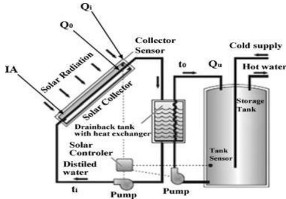
**Figure 2:** A typical active solar thermal storage, (Adapted from Santiago and Jiménez 2002)
