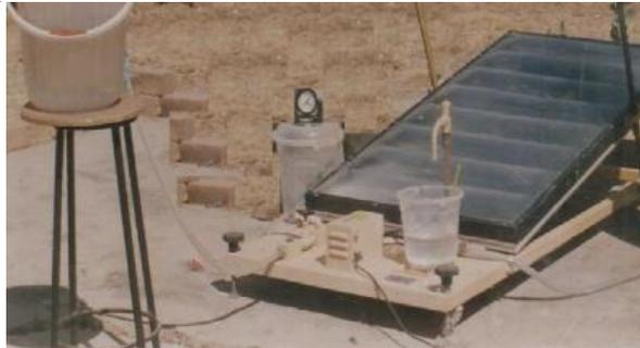
**Figure 10:** Experimental setup for Performance Evaluation of Flat Plate Solar Collector (Model TE 39, (Adapted from Abubakar and Egbo 2014))
