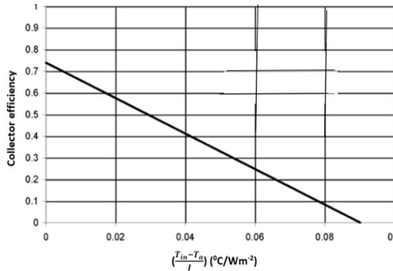
**Figure 12:** Performance of a typical flat-plate thermal collector (ambient temperature 25°C), (Fabio 2008)
