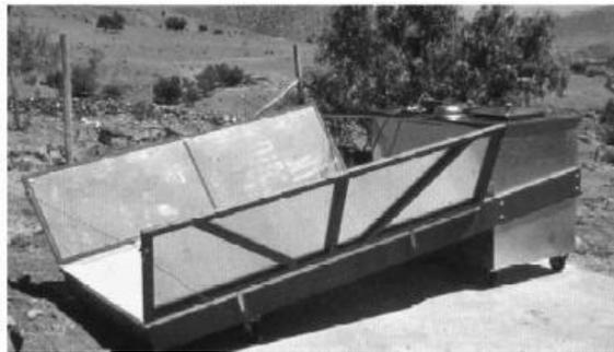
**Figure 11:** Indirect flat plate collector solar cooker with TES, (Adapted from Schwarzer and DaSilva 2003)
