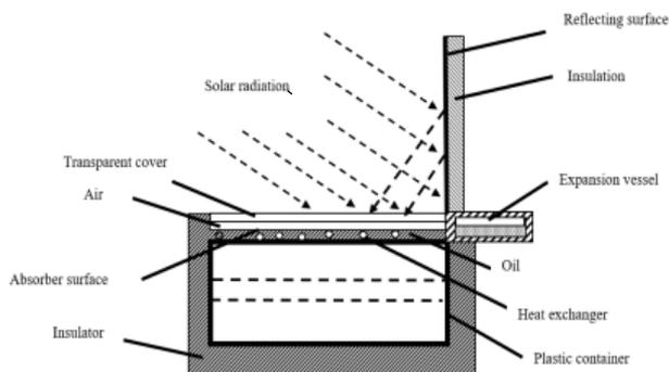
**Figure 8:** Schematic diagram of the integrated solar collector storage system based on a phase-change material, (Chaabane et al 2014).
