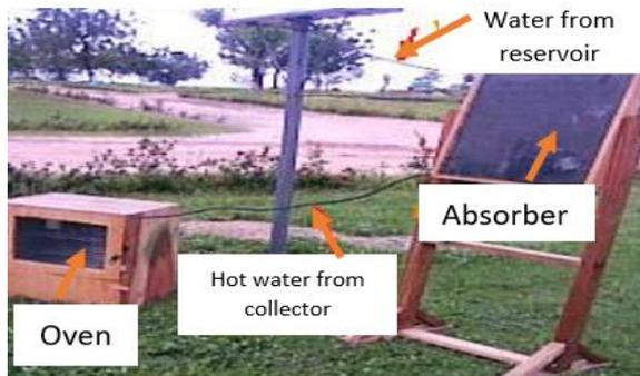
**Figure 13:** Experimental hot water solar oven set up, (Adapted from Bello and Odey 2009)
