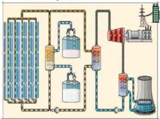
**Figure 3:** Indirect active storage system with 2 tanks, (Adapted from Herrmann and Nava 2006)
