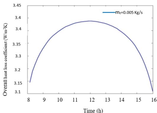
**Figure 15:** Collector overall heat loss coefficient versus time, (Adapted from Hamed et al 2014)
