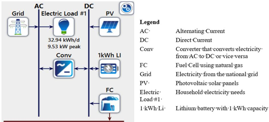
Figure 3: System component design and configuration
