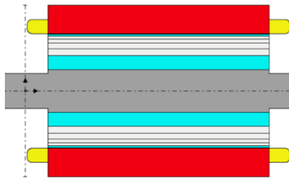
Figure 8: Cross-section view of the motor geometry after obtaining the optimized parameters of the rotor and stator
